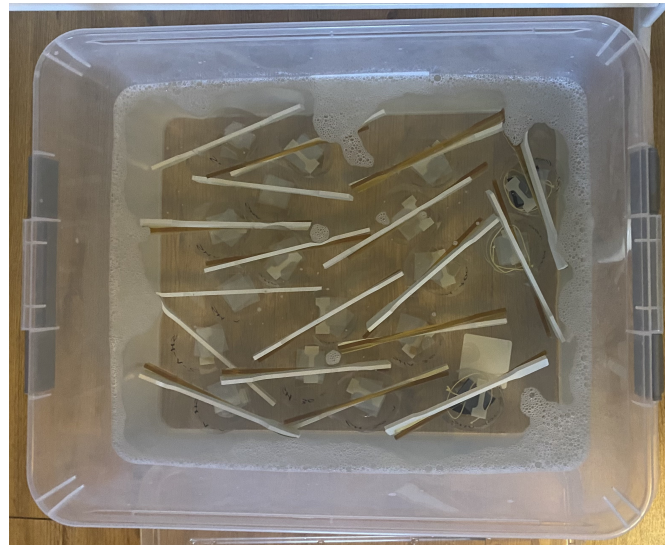
Figure 2.8.: Immersion of samples in 2% glutaraldehyde aqueous solution.
