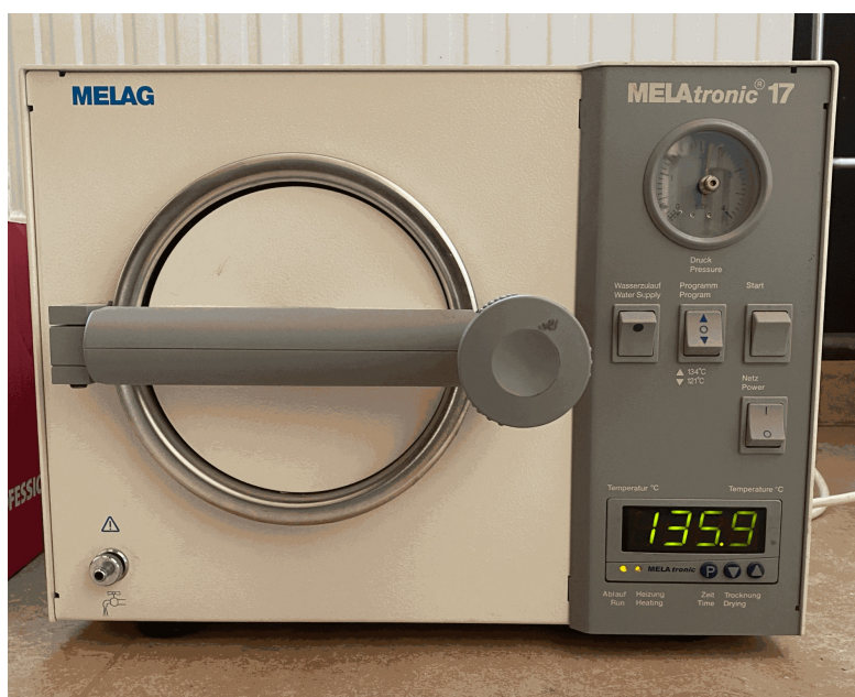
Figure 2.10.: MELAtronic 17 (© MELAG Medizintechnik GmbH & Co. KG) autoclave with pressure gauge and temperature indicator.
