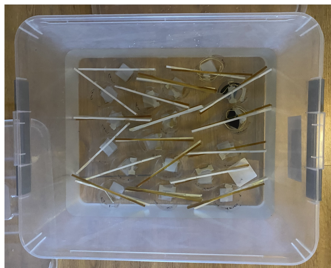
Figure 2.9.: Immersion of samples in 2% sodium hypochlorite aqueous solution.
