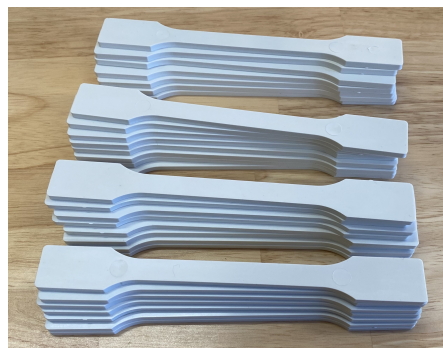
Figure 2.2.: Tensile bars of Grilamid (n=48).
