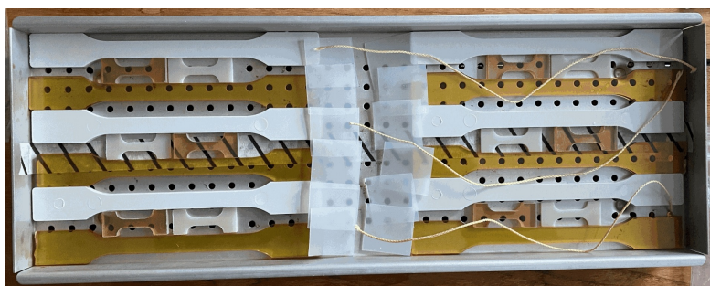
Figure 2.12.: Loaded autoclave tray.
