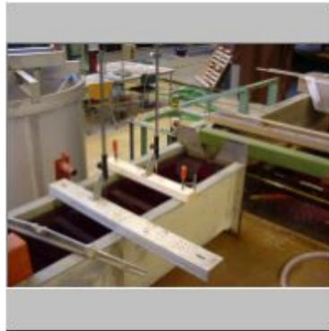
installation of vnotch with good view on vnotch.jpg 303.94 KB
