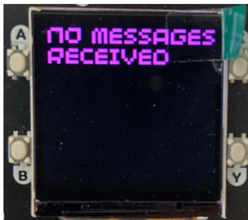
Figure 5: Receive state, no messages received. This screen appears when no message is received for more than 5 consecutive seconds.
