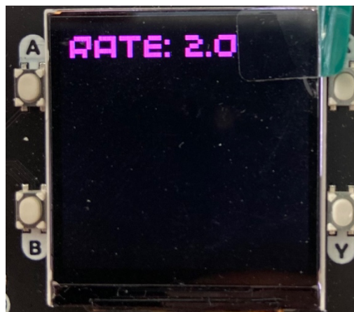
Figure 6: Receive state - rolling window update rate. This is the number of messages correctly received per second averaged over a 5-second interval
