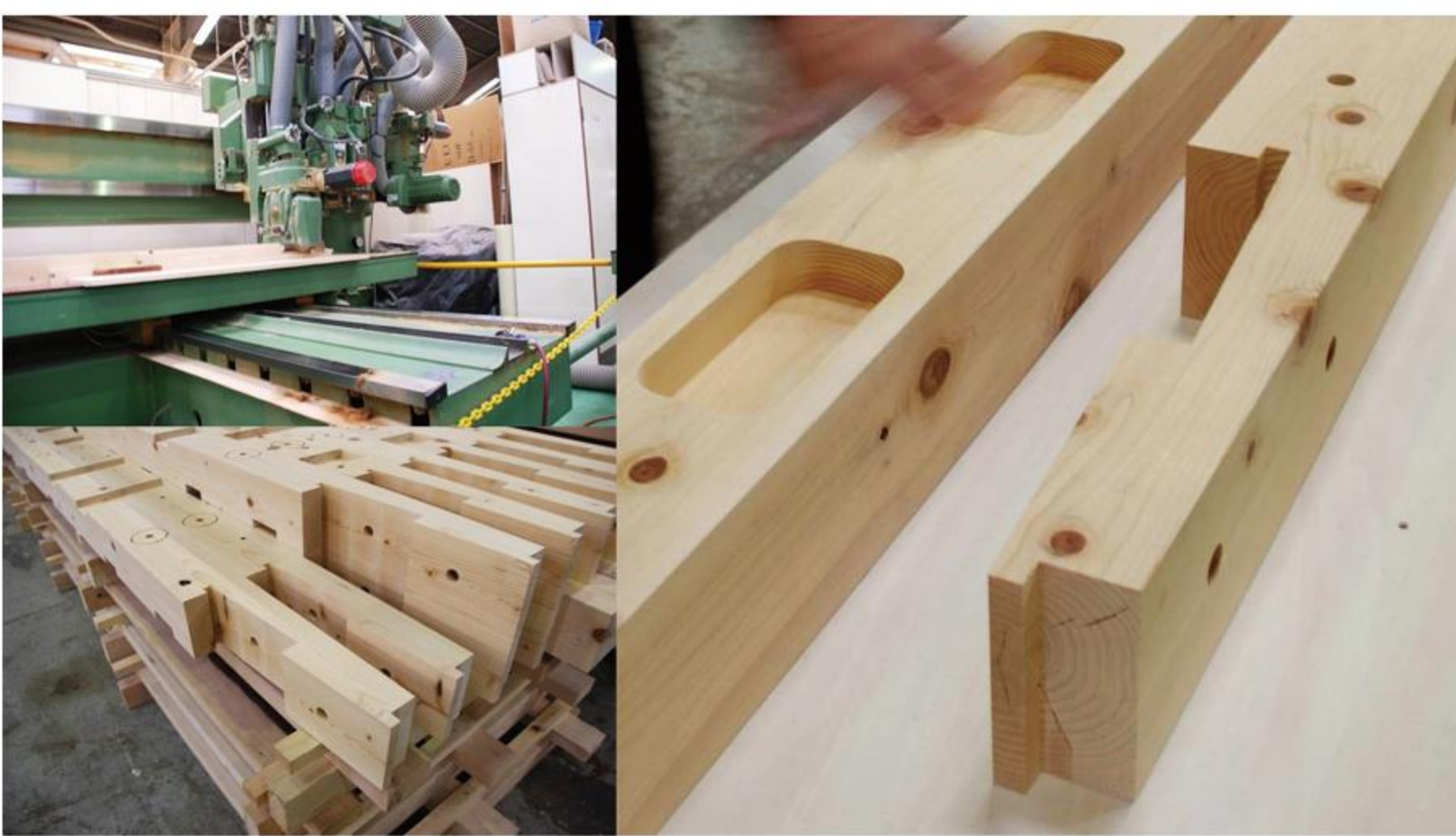
Figure 2. Digital fabrication of timber (Mokuzai Kaikan)
