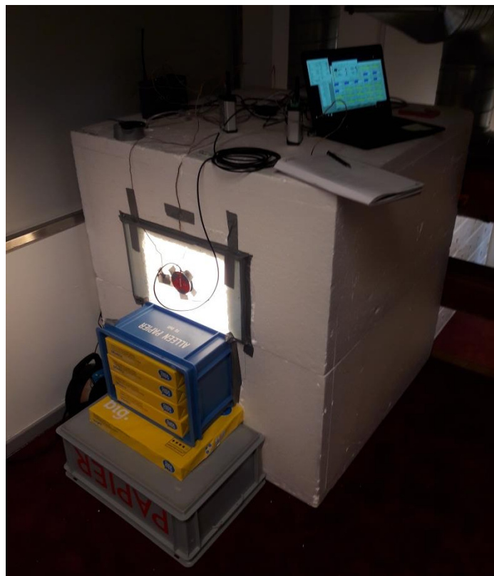
Figure 71 Thermal transmittance test set-up
