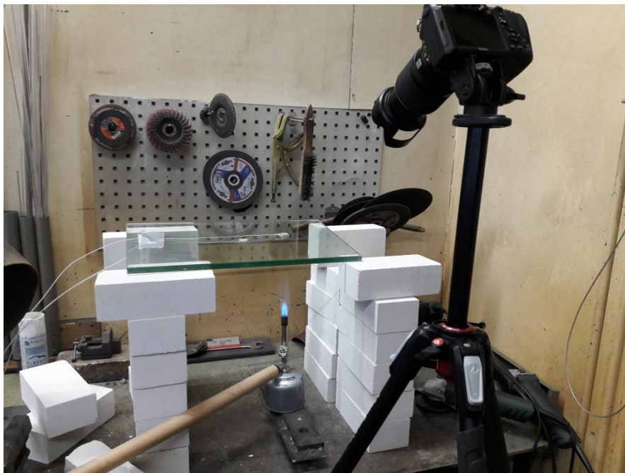
Figure 51 Test set up laminated glass panels with stacked bricks and a burner
