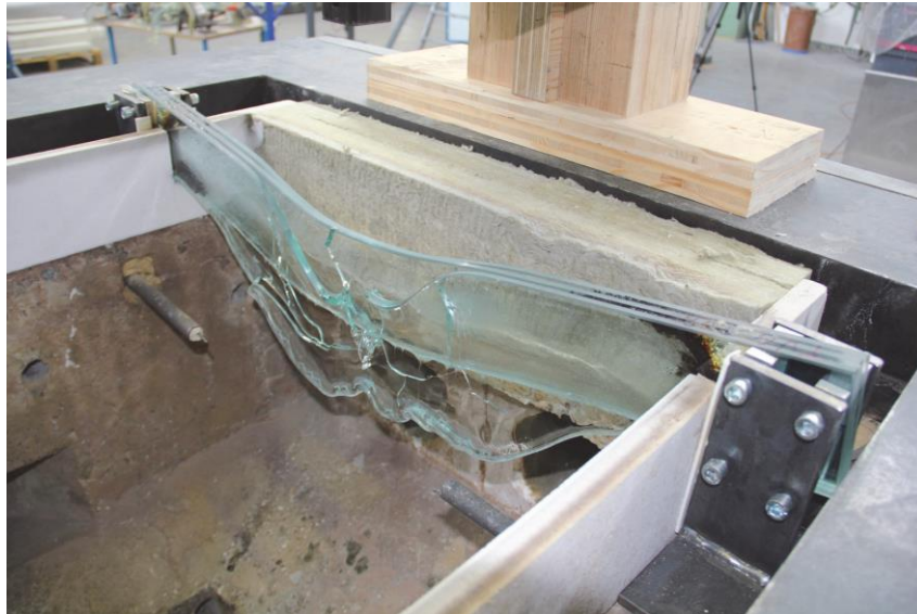
Figure 19 Glass beam with molten mid-span and disappeared PVB interlayer after testing (Louter & Nussbaumer, 2016)
