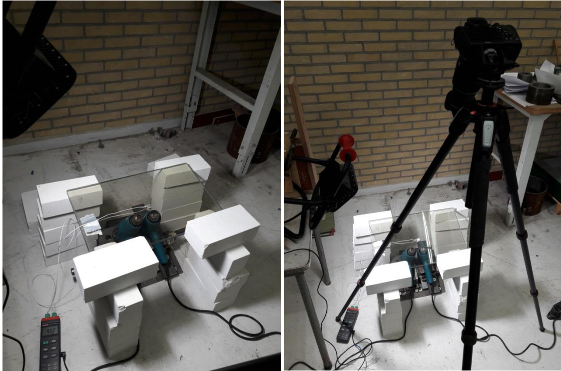
Figure 49 Test set up laminated glass panels with stacked bricks and a heater
