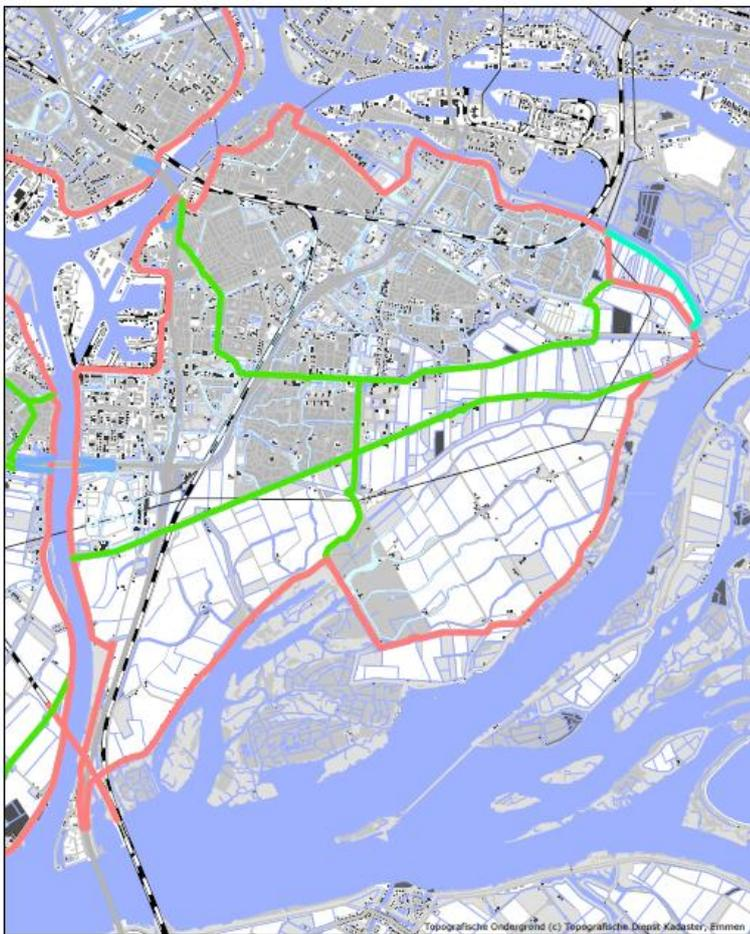
**Figure 6-6: Dike ring 22. Primary flood defenses are indicated in red, secondary flood defenses in green. Parts of the neighboring dike rings are visible. (Source: Waterschap Hollandse Delta)**
