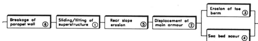
FIG. 11. Decomposition of the fault tree Fig. 8 into series and parallel systems.
