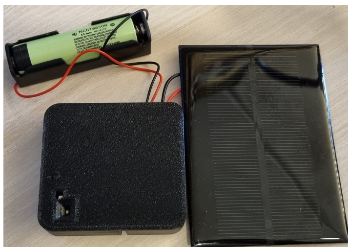
Figure 6.1: An image of how the sensor was deployed during the field tests. The image shows a 3d printed case with holes for the microphone, environmental sensor and light sensor. A 3300 mAh LiPo battery and 110x80mm solar panel are connected to power the ChirpAlert system.
