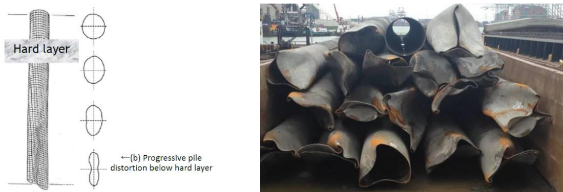
Figure 2.18: Pile tip extrusion buckling. (Randolph, 2018)
