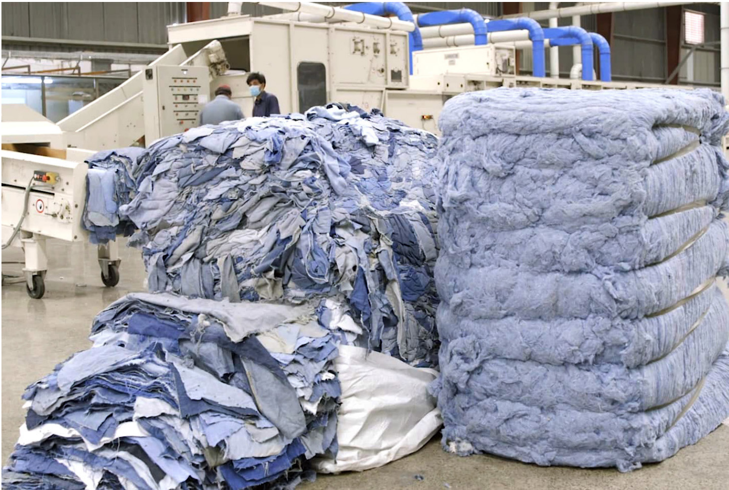
Figure 24. Mechanically recycled denim in different stages of the recycling process
