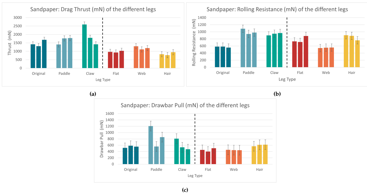
Figure 7.11: Force graphs of each experiment for the different legs on the Sandpaper Surface: (a) Drag Thrust (b) Rolling Resistance (c) Drawbar Pull
