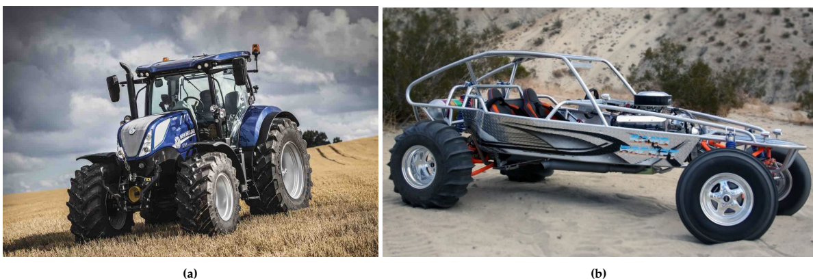
Figure 1.6: (a) Tractor with large wheels and deep treads [24]. (b) Sandrail with front flotation tires and rear paddle tires [25]
