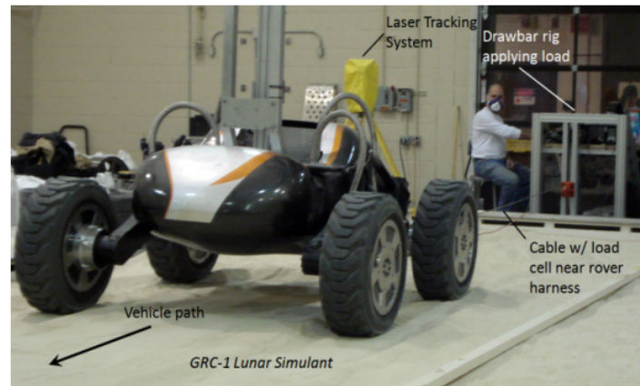
Figure 8.2: Standard Set up for measuring the Drawbar Pull of a vehicle [81]
