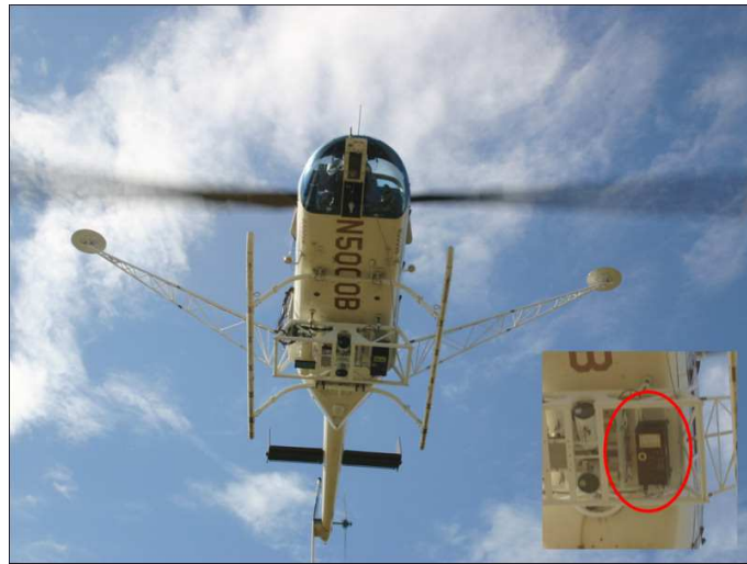
Figure 3.4: The FLI-MAP system [18], the laser scanner is indicated with the red ellipse.
