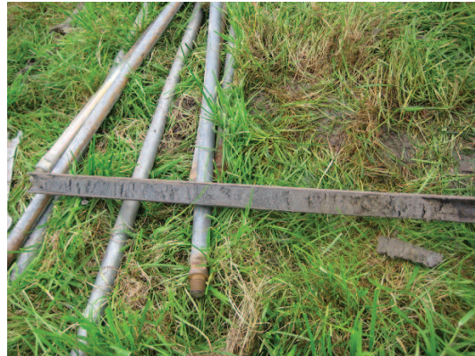
Figure 7.4: Close-up of a gouge used for the drillings. You can see a cross-section of approximately 0.5 m of soil (in this case clay).
