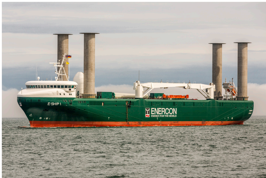
Fig. 1. The E-ship 1 is a wind-assisted ship equipped with four Flettner rotors.
