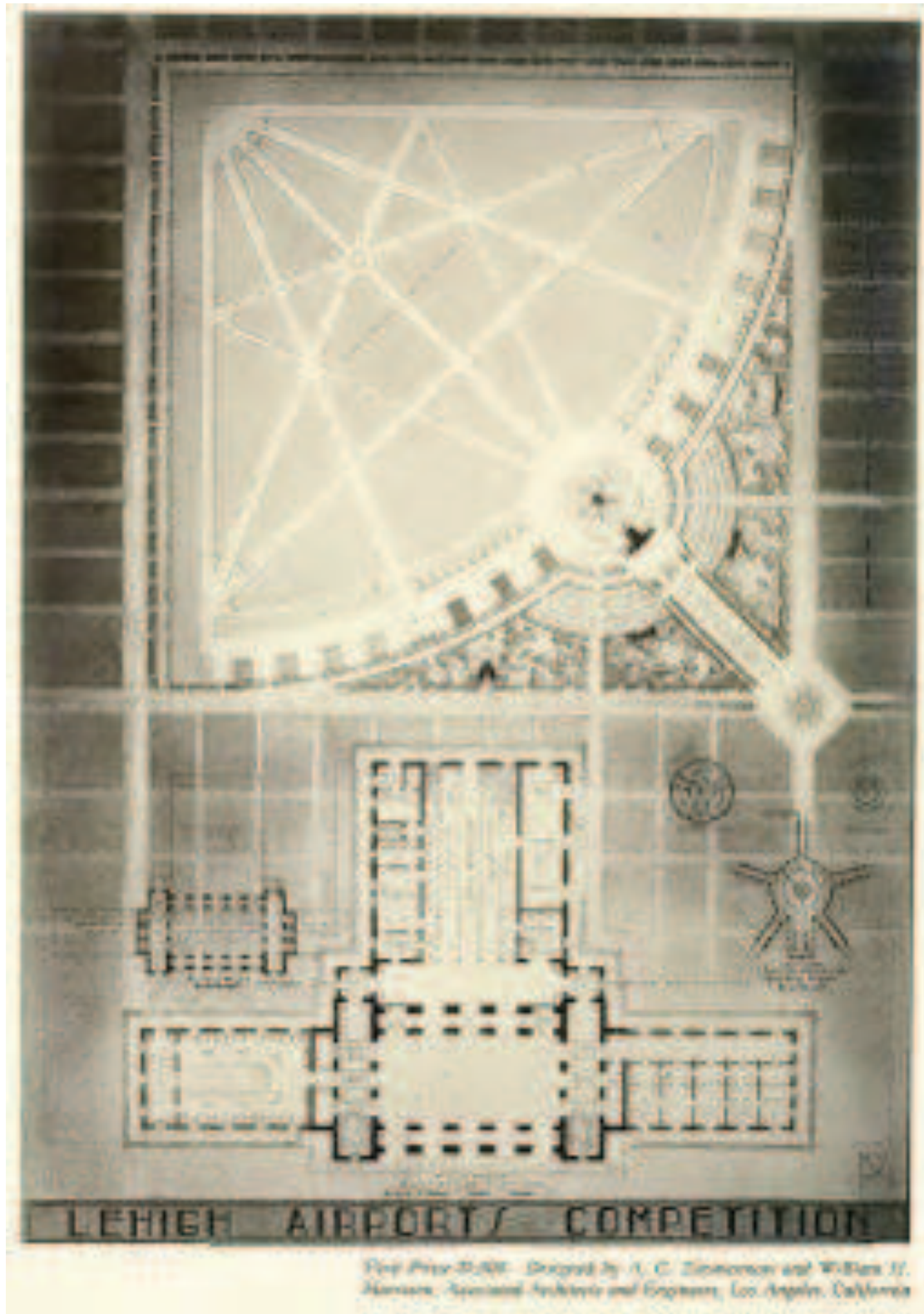
Pic 7: First prize proposal by A.C. Zimmerman and William H. Harrison. Master Plan and ground floor plan of the Air Station and floorplans of the satellite building for boarding on the apron.
