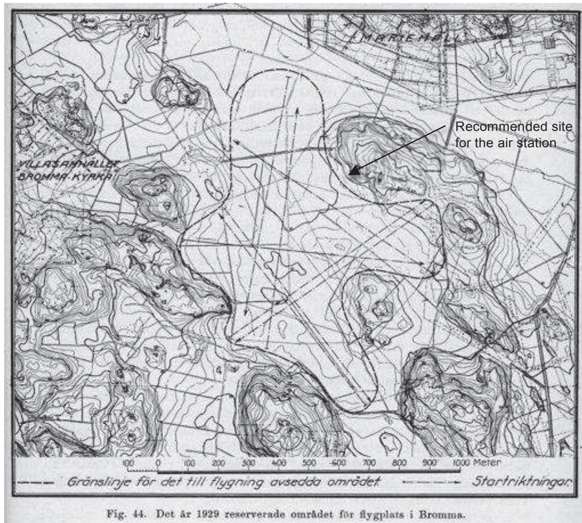
Pic. 13: The Riksby fields in Bromma 1929. The first airport map with the operative borders and eight runway directions marked. The hilly surroundings and the crammed airport field are clearly visible.
