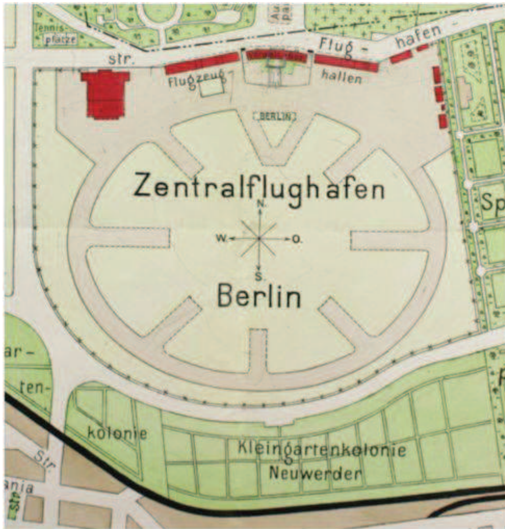
Pic 9: The original Tempelhof field was slightly elliptic with a maximum dimension of 1200 m. The grassfield was surrounded by a paved taxi-way with adjoining start aprons in the field's periphery. Copy of part of a tourist map from the late 1920s.
