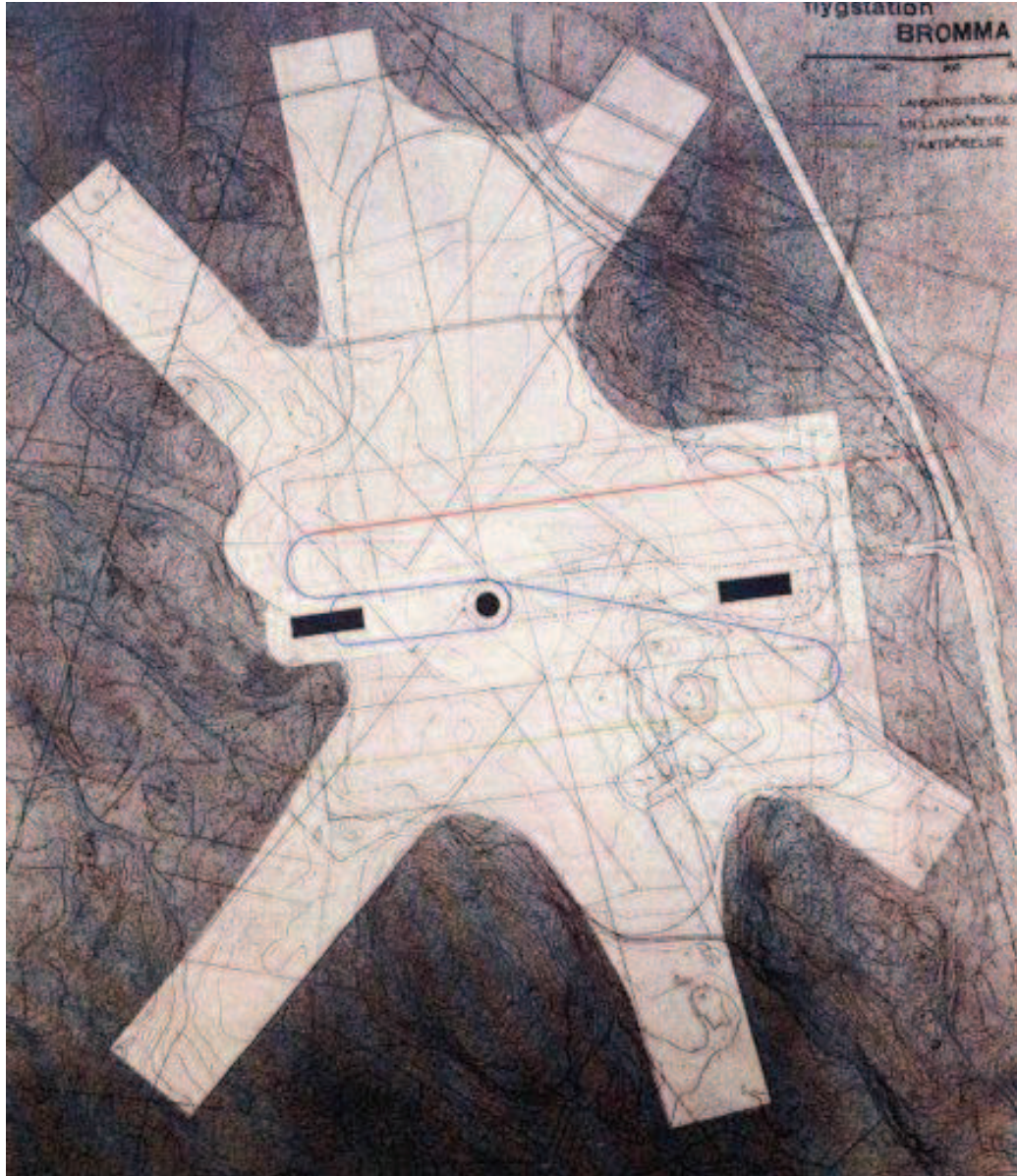
Pic 25: Sven Markelius; Proposed master plan for Bromma airport. Alternative II . Note the marking of separate runways for landings (red) and take off (blue).
