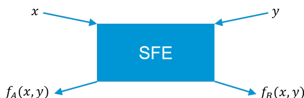
Figure 1.1: Schematic of a general two-party Secure Function Evaluation. At the start of the protocol Alice (left) has an input x and Bob (right) has an input y . At the end, Alice has f_A(x, y) and Bob has f_B(x, y) . Alice does not know more about y than what f_A(x, y) reveals and Bob does not know more about x than what f_B(x, y) reveals.
