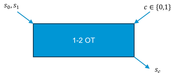
Figure 1.3: Schematic of 1-out-of-2 Oblivious Transfer. Alice (left) gives two messages s_0 and s_1 as input. Bob's (right) input is a choice c \in \{0, 1\} . The protocol outputs only the message of Bob's choice only to Bob.
