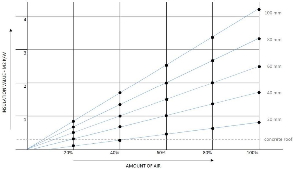
Table 2. Impact of increasing the amount of air in different size of panels on the insulation value (Own work)
