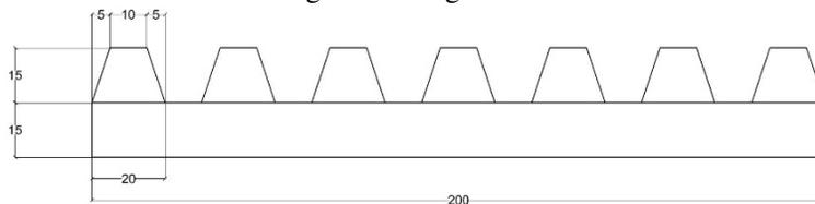
Figure 8. Measurements mold.(Own work)
