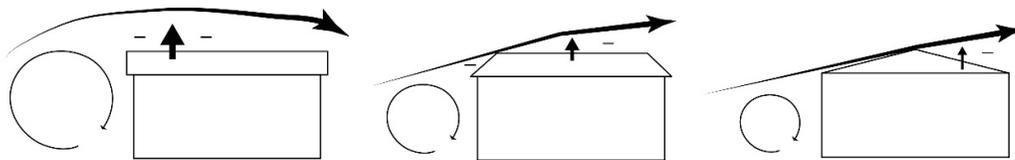
Figure 2. Wind forces on gable, hip and pyramid roof (Own work)
