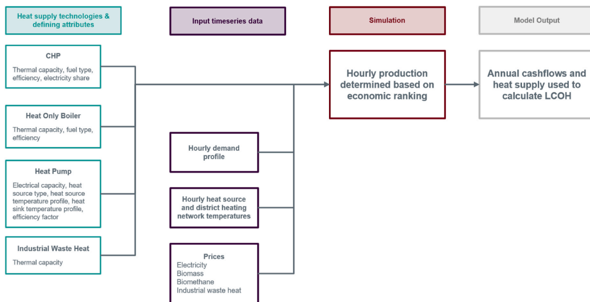
Fig. 2. Overview of TESCA simulation model, accounting for technology configurations, time series data, and deriving model outputs from hourly dispatch simulations.
