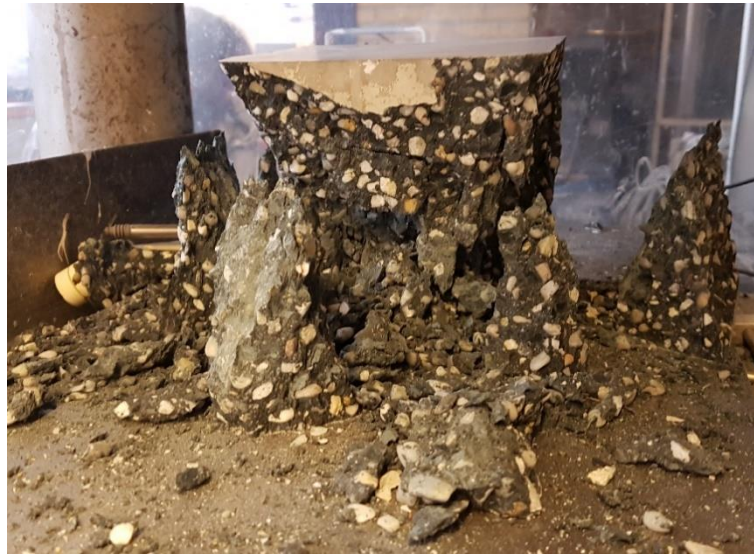
Figure 5.29. Second cubical specimen after failure.
