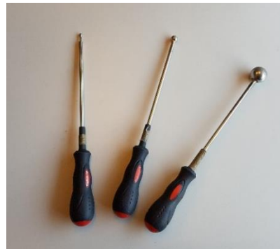
Figure 3.13. Hammers used to create impulse.
