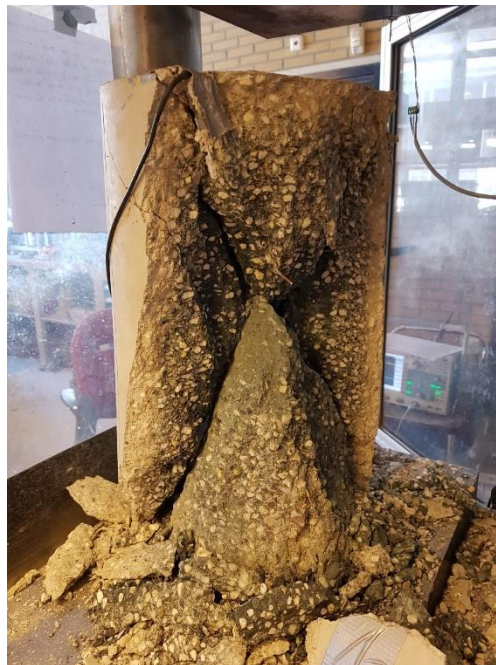
Figure 5.37. First cylindrical specimen after failure.
