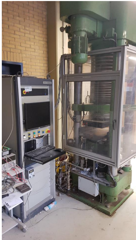
Figure 3.2. Loading apparatus for compression samples.
