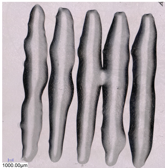
(g) 7 min. precure, printed with snap-off height.
