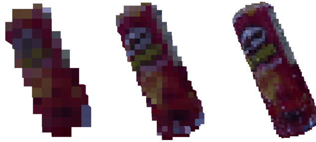
Figure 3-2: Item with voxel size of 2 centimeters (left), 1 centimeter (middle) and 0.5 centimeters (right)
