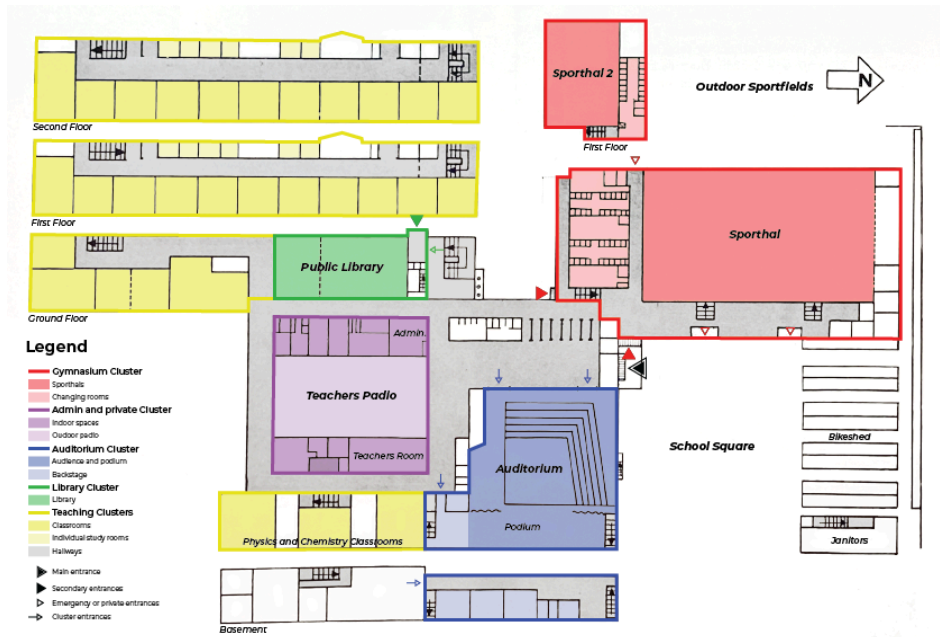
Figure 3.H, The Five Main Functional Clusters of the Rijnlands Lyceum in Oegstgeest, BOUW, 1972 [17] , edits: own work, 2024
