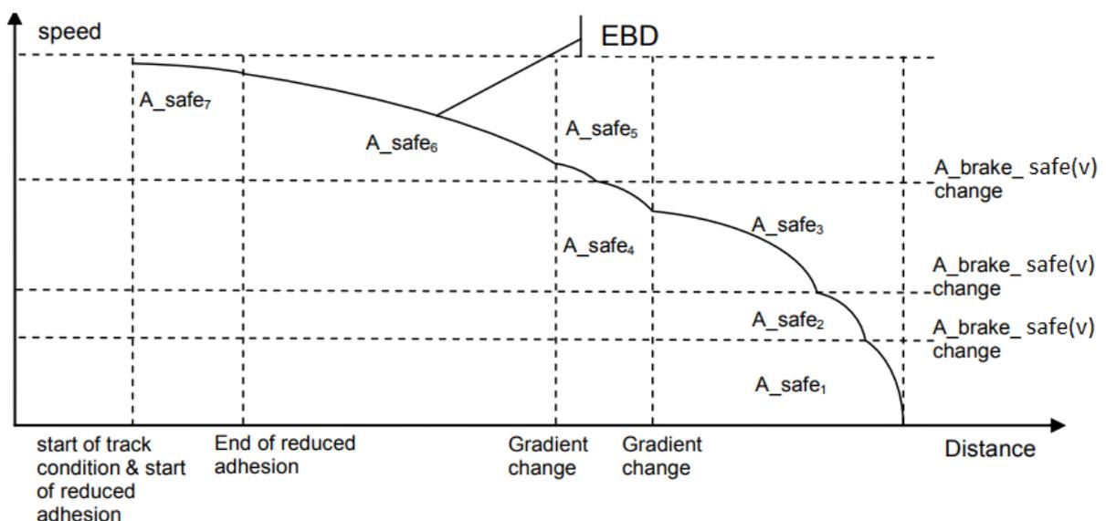
Figure 24 | Construction of the EBD-curve (European Railway Agency, 2016)
