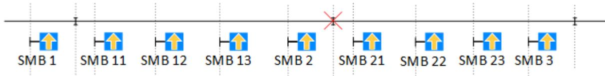
Figure 46 | ERTMS/ETCS Hybrid Level 3 infrastructure model, small virtual subsections, reduced trackside train detection
