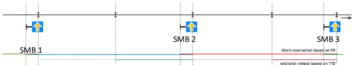
Figure 38 | Infrastructure modelling and block reservation/release of ERTMS/ETCS L2 in RailSys. The colors indicate the reservation and release of the blocks
