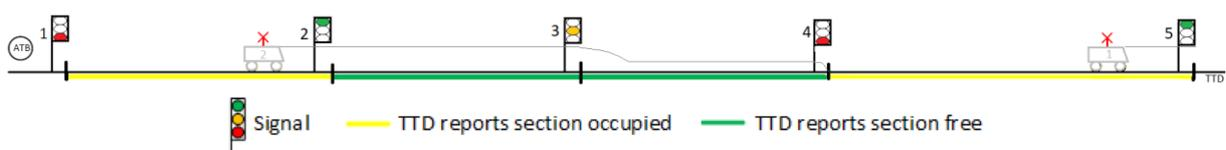
Figure 6 | Train following under NS'54/ATB-EG three aspect signalling
