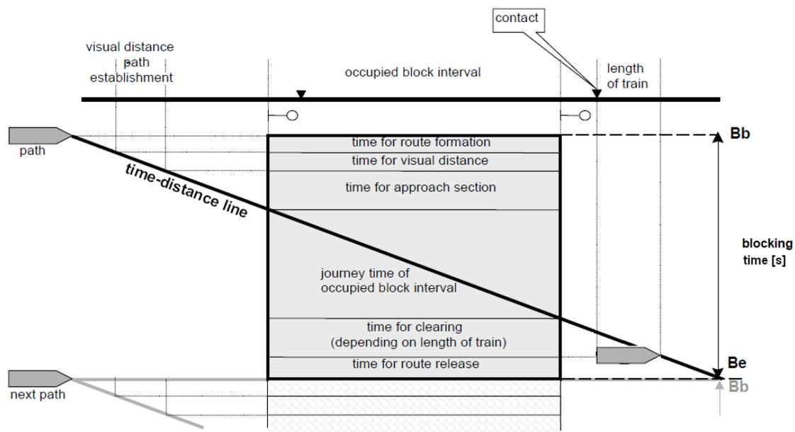
Figure 15 | Single block section – blocking time build up (UIC, 2013a)
