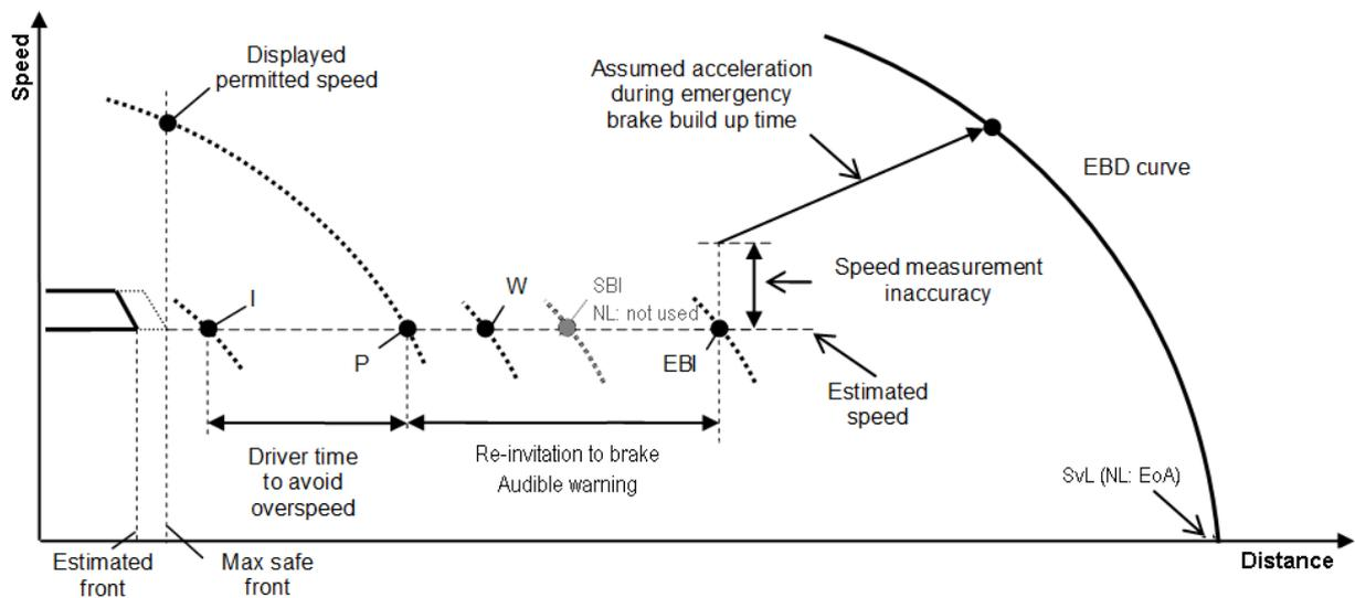
Figure 19 | ERTMS/ETCS braking curves and supervision limits (European Railway Agency, 2016)
