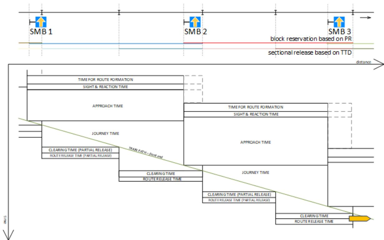
Figure 29 | ERTMS/ETCS Level 2 blocking time diagram
