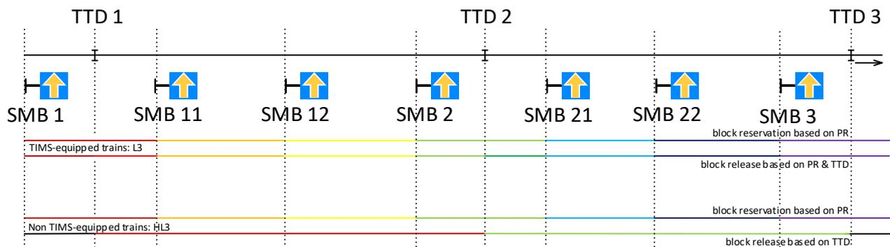
Figure 39 | Infrastructure modelling and block reservation/release of ERTMS/ETCS Hybrid Level 3 in RailSys. The colors indicate the reservation and release of the blocks
