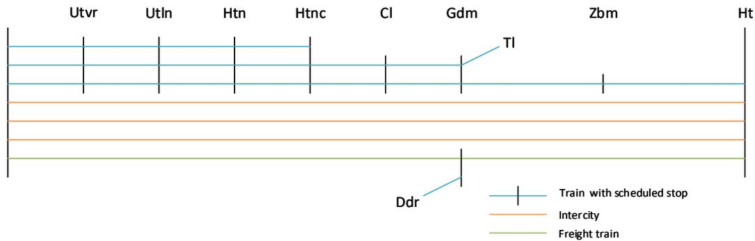
Figure 34 | Schematic overview of the train services, each line represents 2 trains per hour
