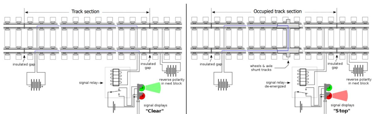
Figure 1 | Track circuits for train detection: track free and track occupied (Wikipedia, 2019a)
