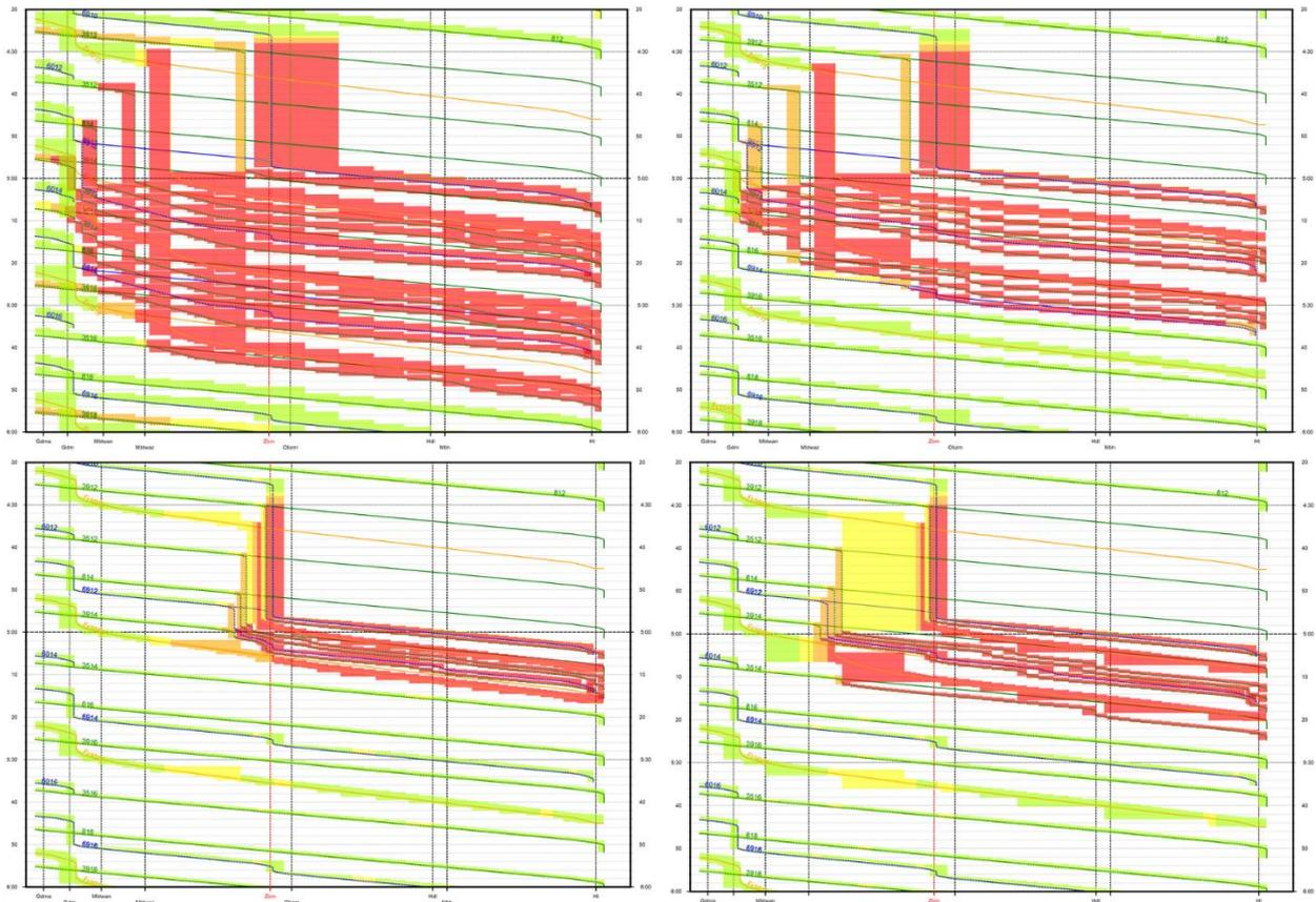
Figure 51 | 30-minute perturbation, Zaltbommel: NS'54/ATB-EG (top left), ERTMS/ETCS L2 (top right), ERTMS/ETCS HL3 with existing TTD (bottom left), ERTMS/ETCS HL3 with reduced TTD (bottom right)
