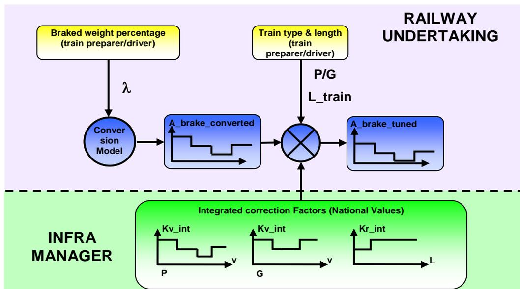
Figure 22 | Lambda braking: Conversion Model & Integrated Correction Factors (European Railway Agency, 2016)
