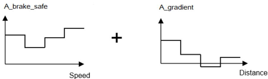
Figure 23 | Composition of  $A_{safe}$ :  $A_{brake\_safe} + A_{gradient}$  (European Railway Agency, 2016)
