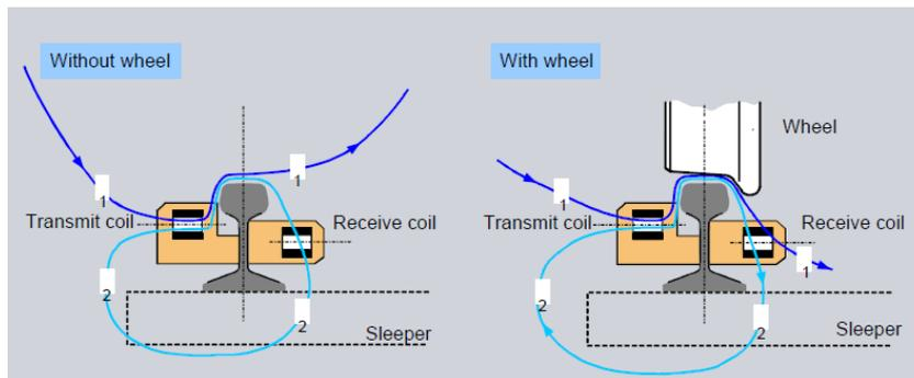
Figure 2 | Axle counters for train detection: track free and track occupied (RailSystems.net, 2019)
