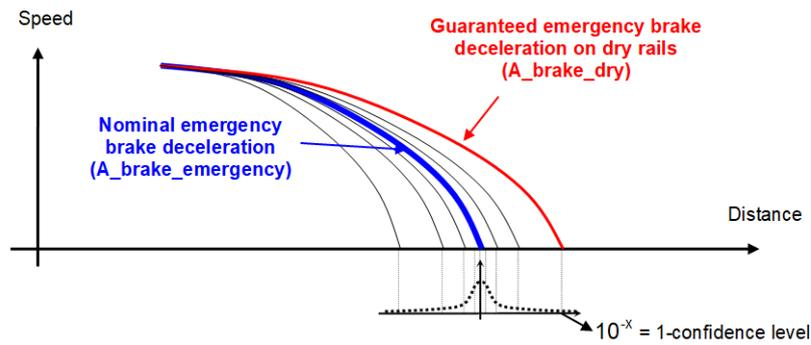
Figure 20 | Dispersion of emergency braking performance (European Railway Agency, 2016)
