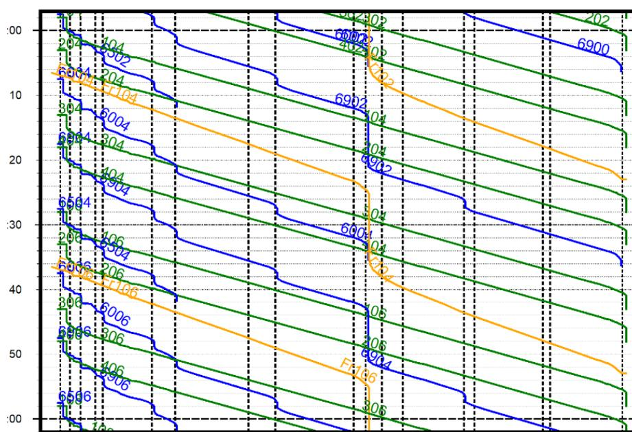
Figure 55 | Pattern of the extended simulated timetable: 8 ICs/hour
