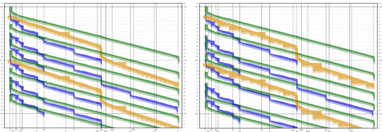
Figure 50 | Compressed timetables for HL3 with existing TTD (left) and HL3 with reduced TTD (right) including 60 seconds buffer time per train
