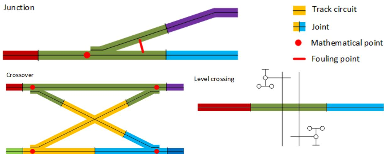
Figure 58 | Projection of track circuits on junctions, crossovers and level-crossings (ProRail, 2012)
