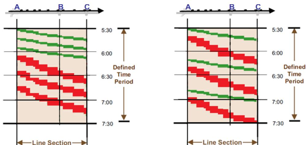
Figure 17 | Track occupation for homogeneous and mixed traffic (UIC, 2013a)
