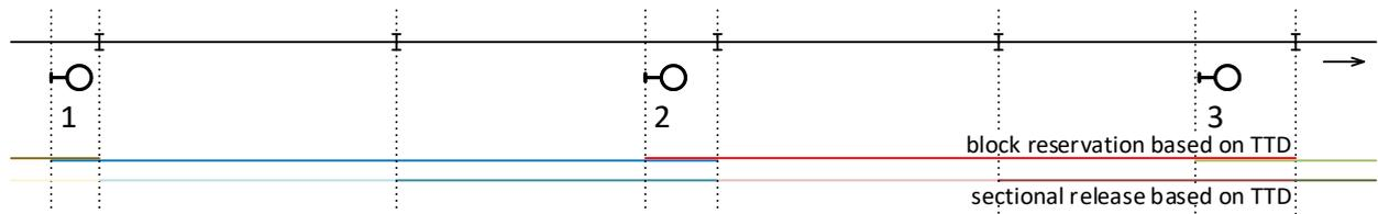
Figure 37 | Infrastructure modelling and block reservation/release of NS'54/ATB-EG in RailSys. The colors indicate the reservation and release of the blocks
