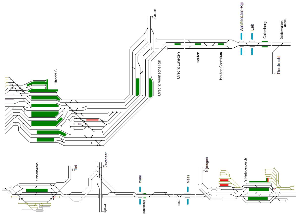
Figure 33 | Schematic overview of the track layout Utrecht - Den Bosch (Sporenplan, 2018)
