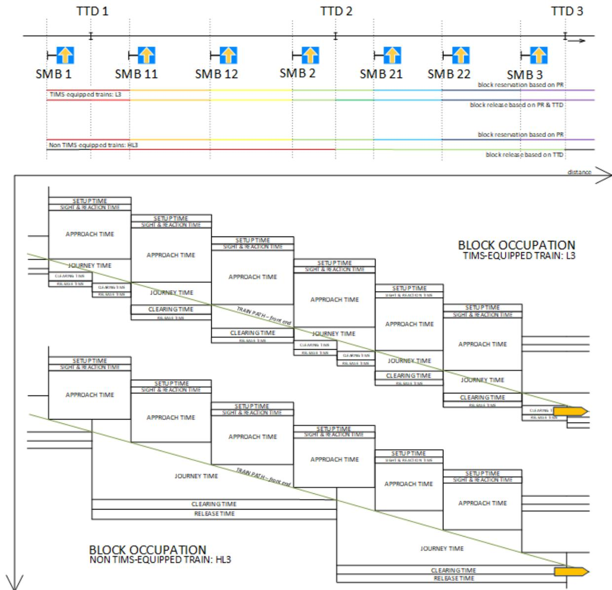
Figure 30 | ERTMS/ETCS Hybrid Level 3 blocking time diagram
