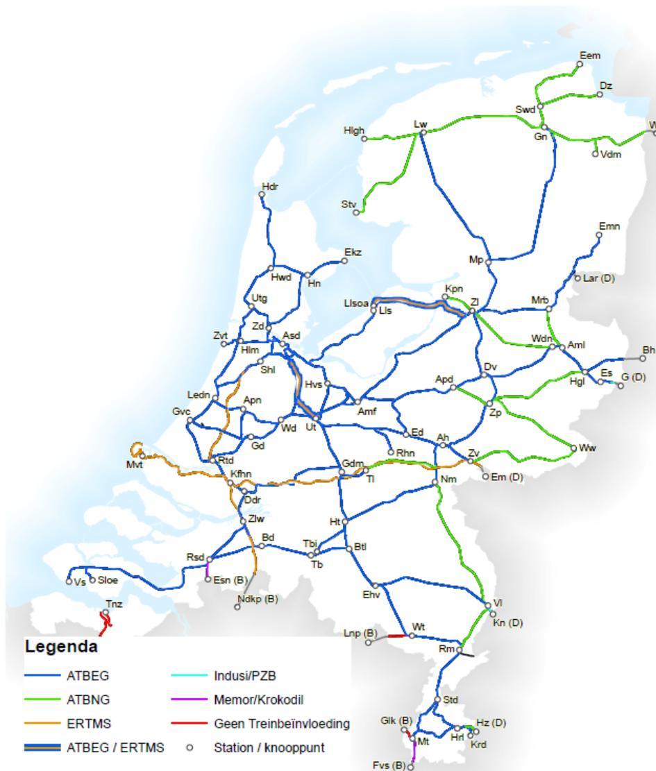
Figure 3 | Automatic Train Protection systems on the Dutch network, situation 2018 (ProRail, 2018a)
