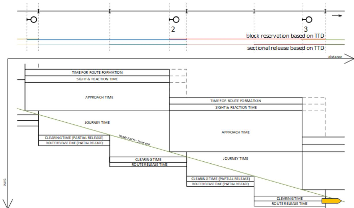
Figure 28 | NS'54 / ATB-EG blocking time diagram
