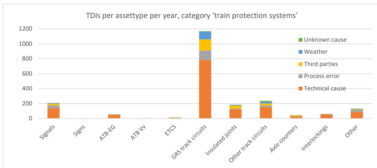
Figure 60 | Break down of the 2018 TDIs in the category 'Train protection systems' (ProRail, 2019b)
