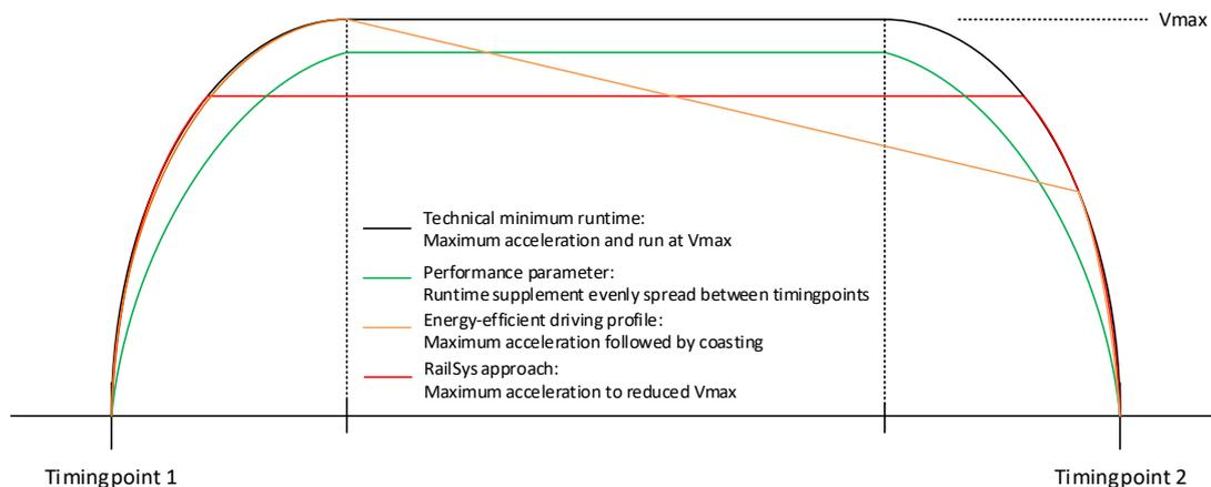
Figure 41 | Different approaches of runtime supplement
