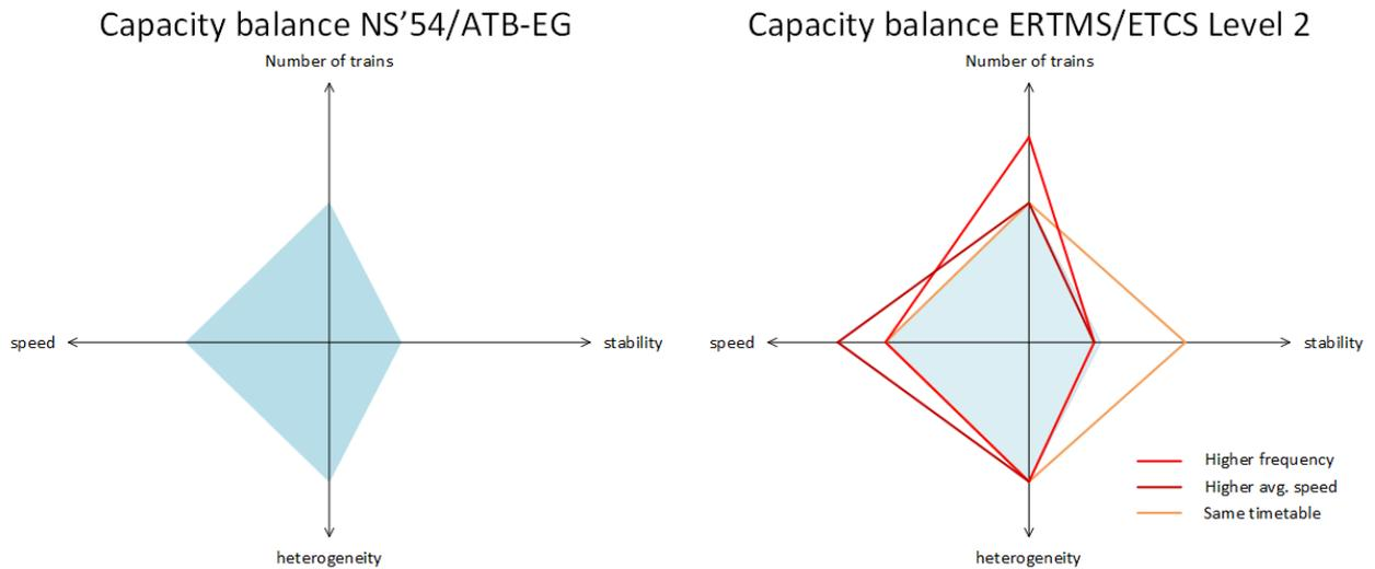
Figure 31 | Change in capacity balance under ERTMS/ETCS Level 2: three scenarios
