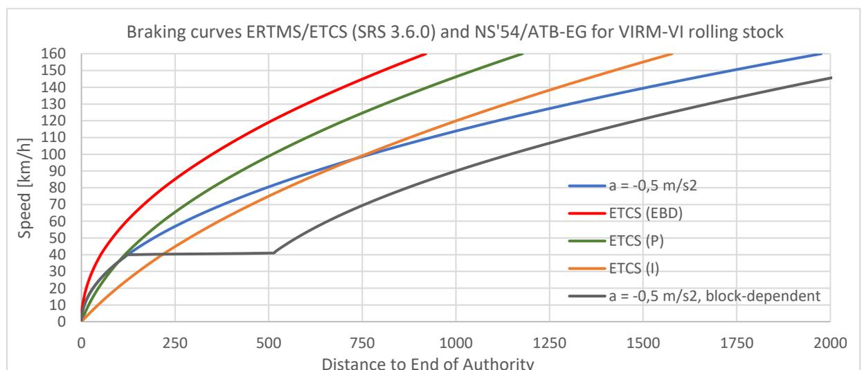
Figure 26 | ATB-EG curve, ATB-EG block-dependent curve and the ETCS-curves (EBD, P, I)
