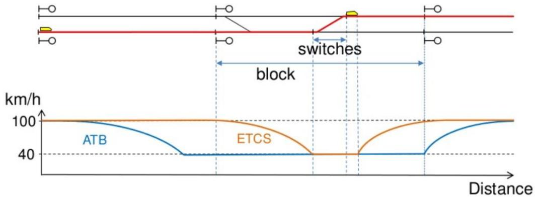
Figure 18 | Block independent and route dependent, train dependent, speed dependent braking under ERTMS/ETCS compared to NS'54/ATB-EG (Goverde, 2018)
