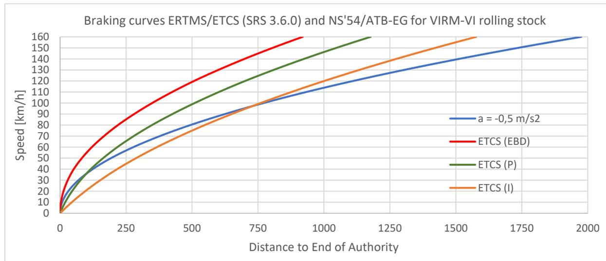
Figure 25 | ATB-EG curve and the ETCS-curves (EBD, P, I) according to SRS3.6.0 (ERTMS User Group, 2016)
