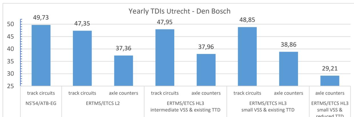
Figure A.1 | Yearly TDIs related to signalling and train protection systems, corridor Utrecht - Den Bosch
