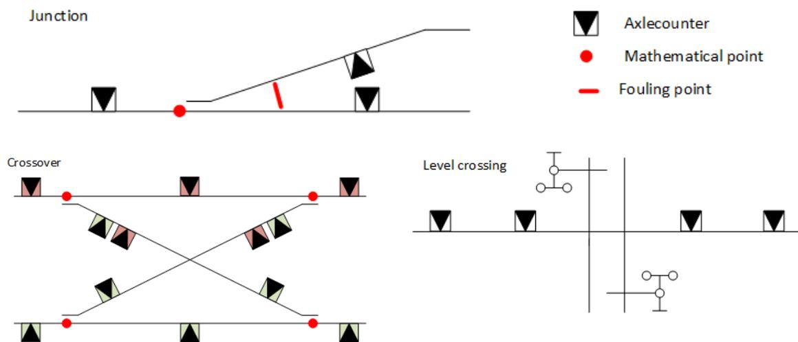
Figure 59 | Projection of track circuits on junctions, crossovers and level-crossings (ProRail, 2018d)
