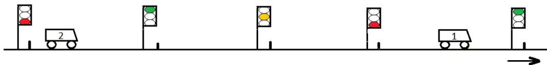
Figure 4 | NS'54 2-block 3-aspect signalling
