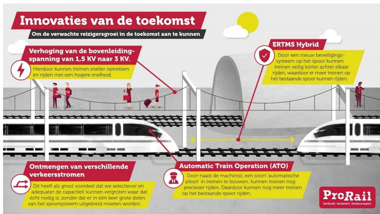
Figure 57 | Future innovations to facilitate railway growth: 3kV, ATO, ERTMS/ETCS and unbundling (ProRail, 2019)
