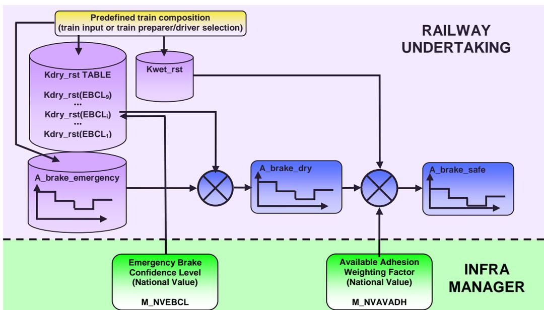
Figure 21 | Gamma braking: braking characteristics & correction factors (European Railway Agency, 2016)
