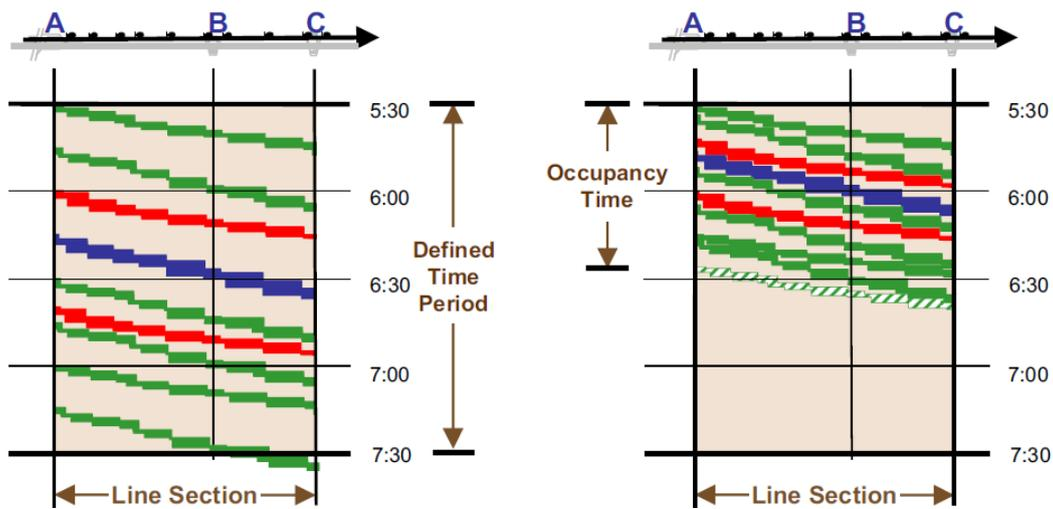
Figure 16 | Blocking time diagram, before and after compression (UIC, 2013a)
