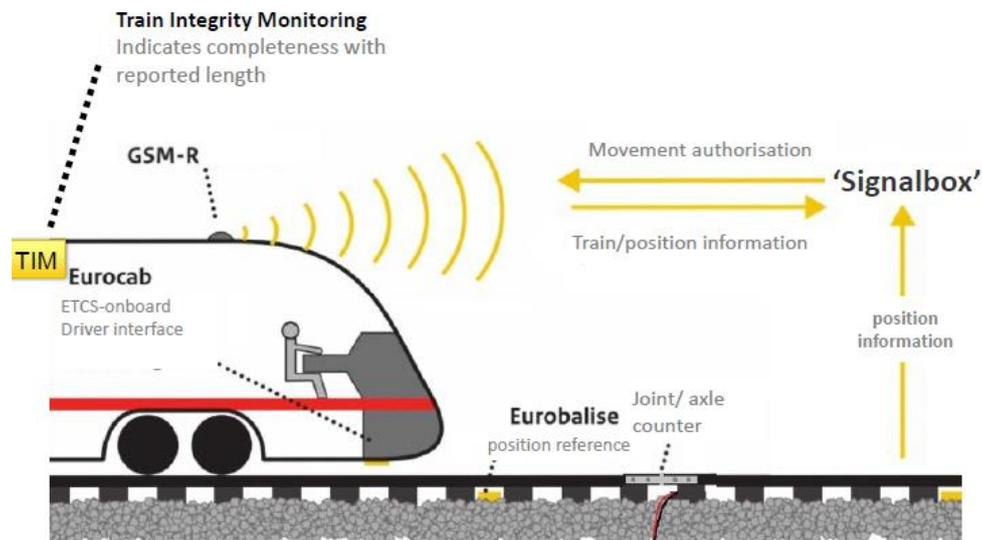
Figure 13 | ERTMS/ETCS HL3 setup
