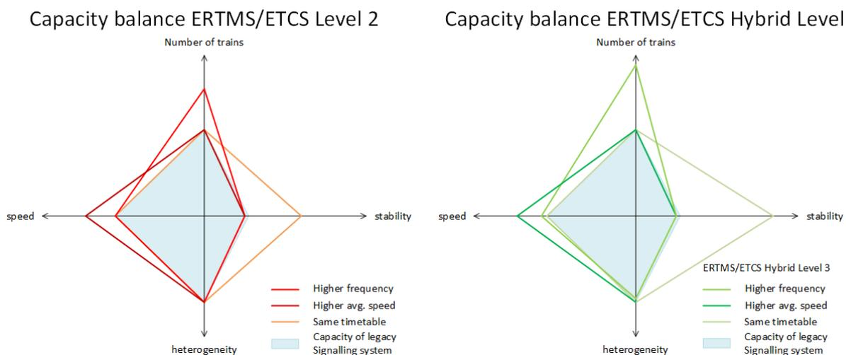
Figure 54 | Capacity balance ERTMS/ETCS Level 2 and ERTMS/ETCS Hybrid Level 3
