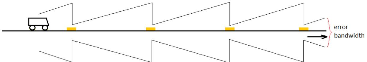
Figure 9 | Train localisation using Eurobalises and onboard odometry. Train location within confidence interval
