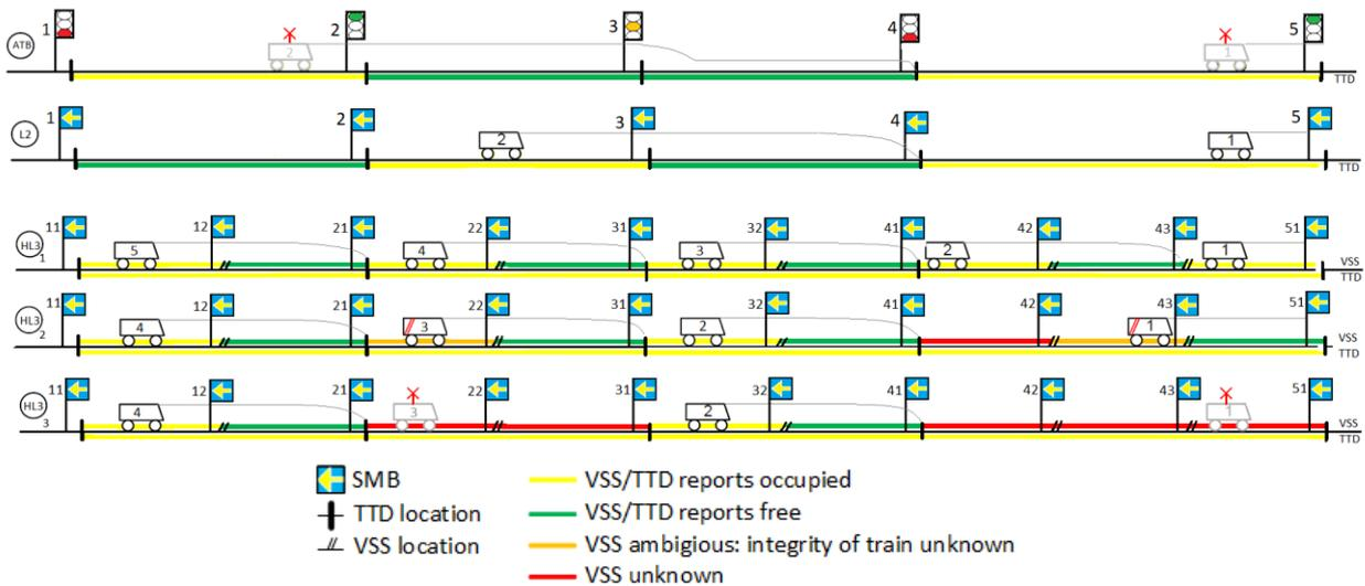
Figure 14 | Train following under ERTMS/ETCS HL3 compared to ATB-EG and ERTMS/ETCS L2
