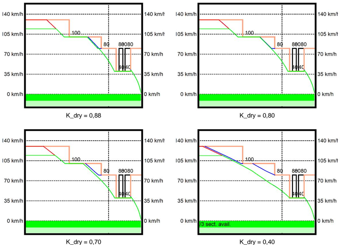
Figure 52 |  $K_{dry}$  influence on the ETCS braking curve, series 6900 train
