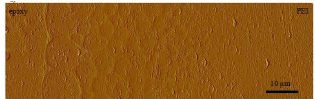
Figure 1.8: AFM phase image of epoxy (tetraglycidyl diaminodiphenyl methane (TGDDM), diglycidyl ether of bisphenol F and triglycidyl-p-aminophenol with diaminodiphenyl sulphone (DDS) hardener) co-cured with PEI. Image from [29].
