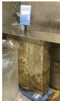
Figure 2.5: Water immersion container with automatic temperature control.
