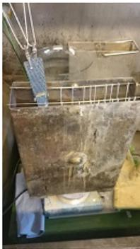
Figure 2.4: Water immersion container with immersed samples.
