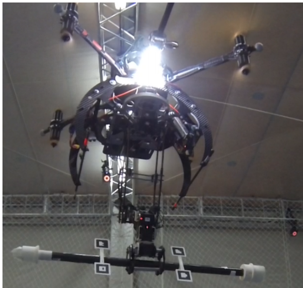
Figure 7: Grabbing a bar with visual markers.
