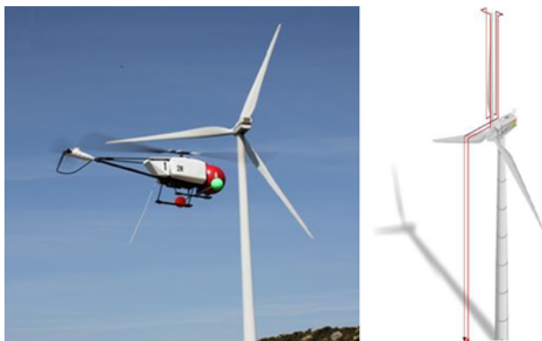
Figure 10: UAV flights close to the wind turbine to be inspected (left); Trajectory followed for the inspection (right).
