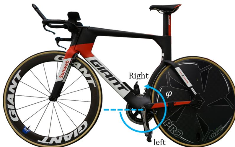
**Fig. 5** Bike crank angle convention.
