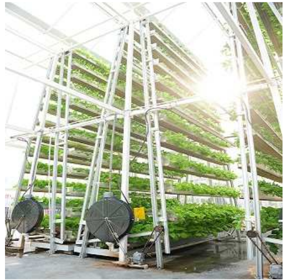
Figure 18. The vertically rotating A-shaped steel frames carrying hydroponic racks filled with leafy vegetables (Singapore Ministry of National Development, 2013).
