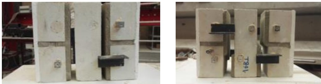
Figure 61 – Typical crack patterns observed during the shear-compression tests on triplets.
