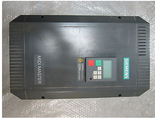
Figure 3.9: MIDI master, actuator frequency regulator
