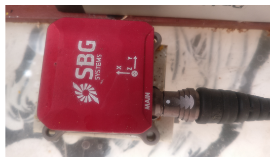
Figure 3.6: Accelerometer, one attached at the bucket and one at the frame, both aligned such that x-direction points in direction of motion.
