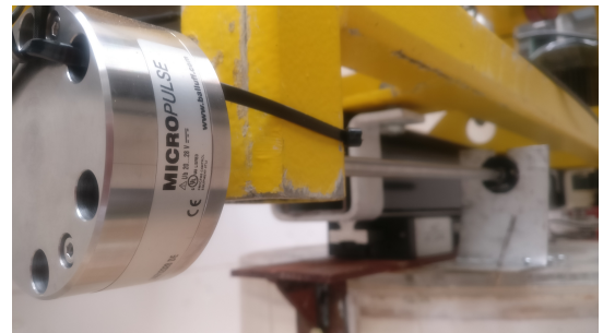
Figure 3.5: BTL sensor, with magnet (in black)
