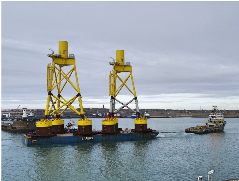
Figure 1.2: Suction Bucket Jackets on transport
