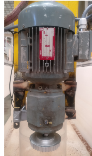
Figure 3.7: Actuator for the forced oscillation (1.5kW).
