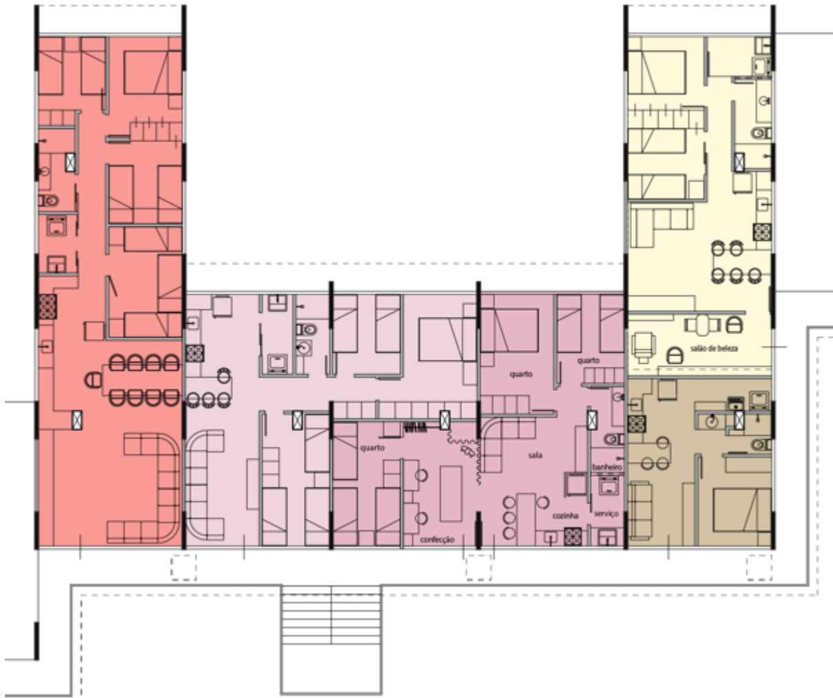
Figure 19: Floor of a base-building part with infill Source: Lamounier, 2017.
