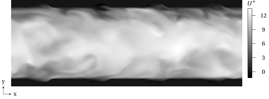
Figure 5.13: Instantaneous snapshot of the velocity field in the streamwise direction ( U^+ ) for the highest-performing dimpled surface of the second generation of the reinforcement learning study at Re_\tau = 180 . The slice shown corresponds to the plane at z = L_z/2 . Please note that U = U^+ in our numerical framework. The bulk flow moves from left to right.
