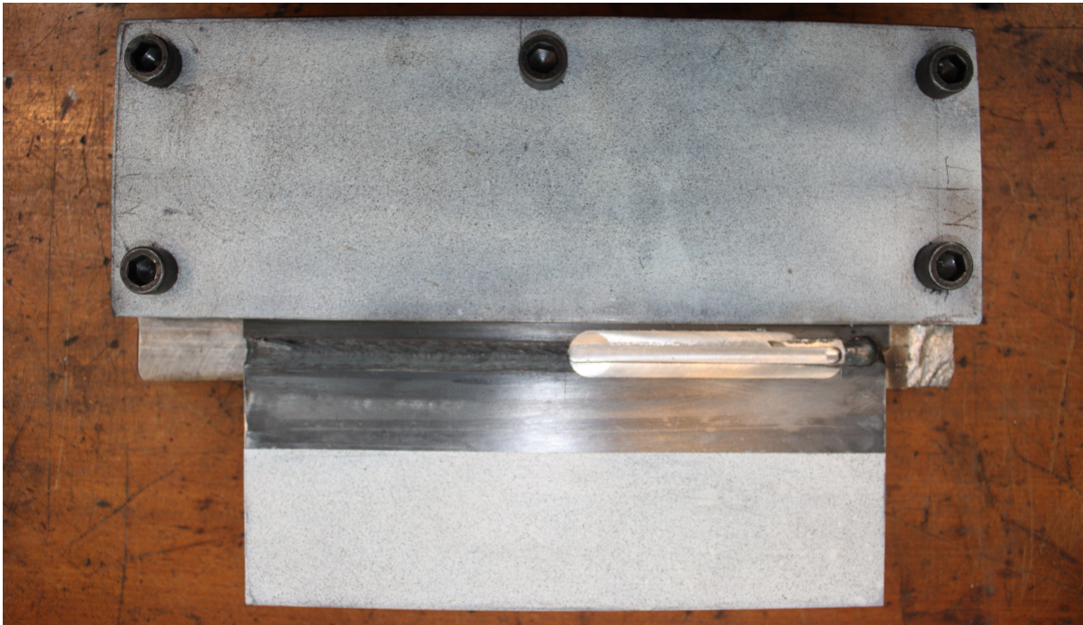
Figure 7.2: Photo of the removed section of the plates. The initial weld was performed from the right to left side of the plate.
