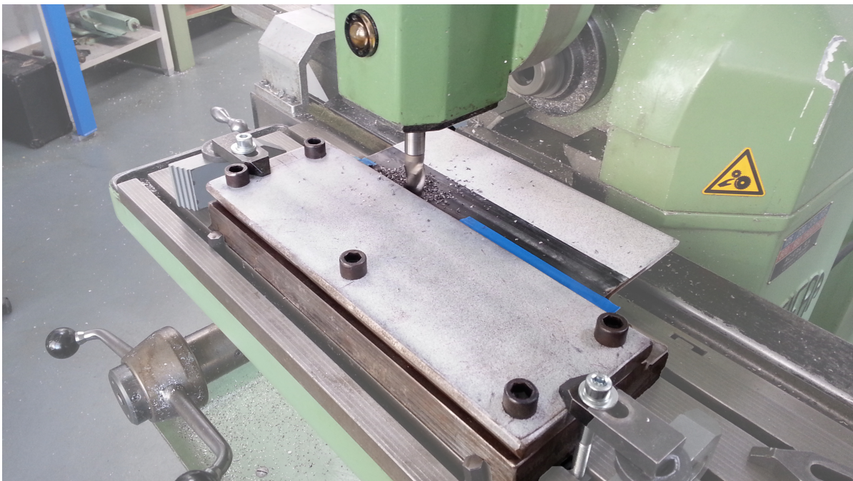
Figure 7.3: Photo of the removal of the section by the milling process.
