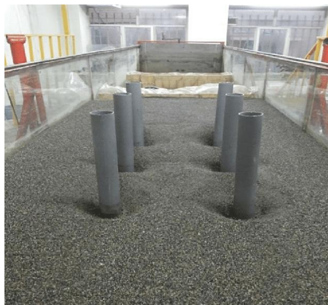
Figure 4.3: Scour holes in a test setup [Amini & Solaimani, 2017]
