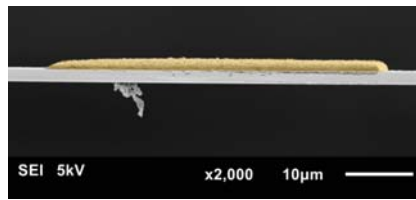
Figure 6.11: An SEM image of a second sample with a polymeric layer near the tip of a cantilever can be seen in this figure. Its thickness is smaller than that of the cantilever. Contamination on the bottom side of the cantilever is revealed by this picture.
