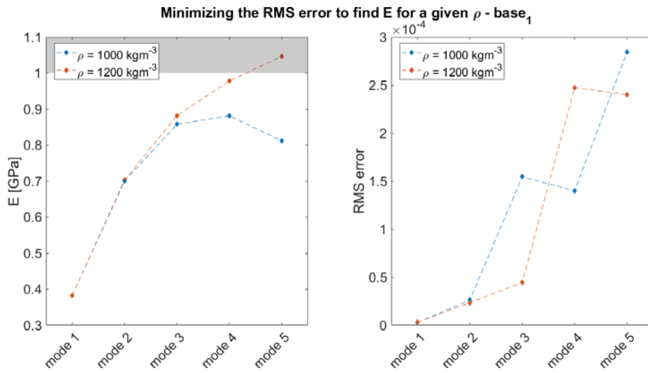
Figure 6.21: In the left graph, the values for E can be obtained from corresponding densities of 1000 \text{ kgm}^{-3} (blue line) and 2000 \text{ kgm}^{-3} (orange line) per mode. The grey area represents the values from literature. The minimum difference found on the experimental and theoretical values are shown in the graph on the right.
