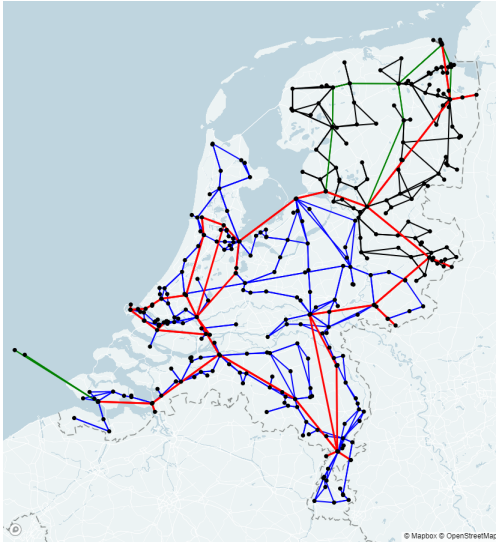
Fig. 1. Dutch high-voltage power grid in 2021 as modelled in pandapower. Prints use map data from Mapbox and OpenStreetMap and their data sources. Black, blue, green, and red lines represent the 110 kV, 150 kV, 220 kV, and 380 kV level, respectively.
