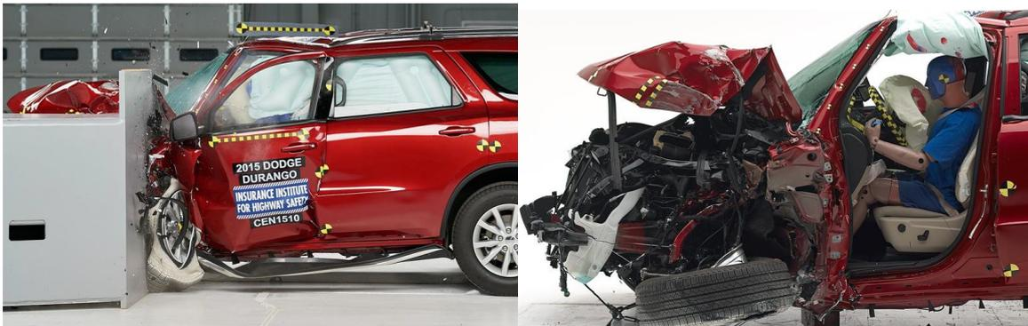
Figure 2.2: *Crash-test results of a 2017 Dodge Durango SUV during a small-overlap frontal crash[19].*
