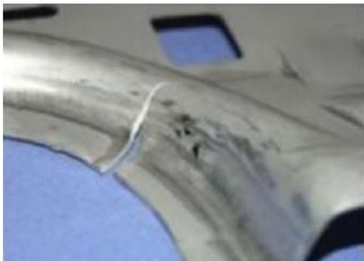
(a) Edge-cracking after forming
