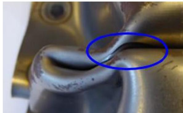
(b) Cracking after folding of a crash-rail
