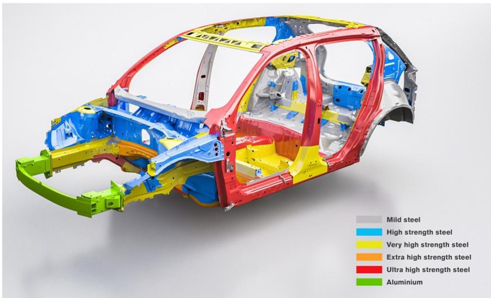
Figure 2.3: Architecture of a 2018 Volvo XC40 cross-over, which was awarded 5 stars in Euro NCAP (highest score) due to its effective use of Ultra High-Strength Boron steel in the safety cage. Image courtesy of Volvo Cars, Sweden.
