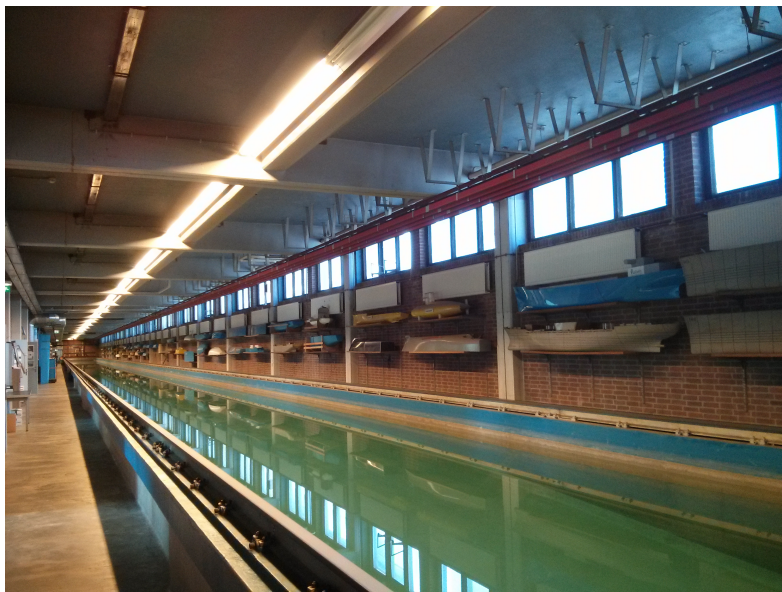
Figure 3.1: Towing tank Nr. 1 of the Delft Ship Hydromechanics Laboratory
