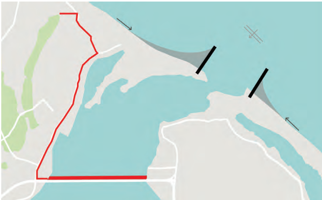
Figure 8.5: Visual impression of Variant D, two jetties to prevent sedimentation in the inlet and a storm surge barrier to prevent flood waves from the sea.
