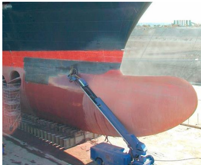
Figure 5-22 An example of bulbous bow
