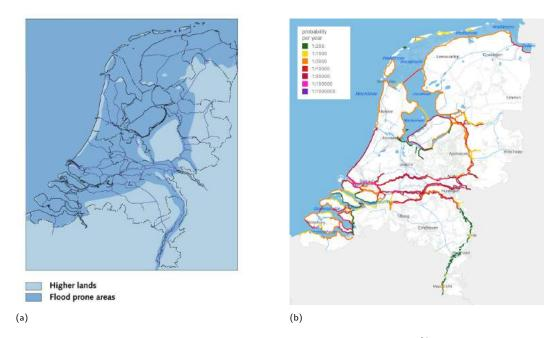
Figure 2.3: Left, the flood prone areas in the Netherlands covering approximately 55% of the Netherlands. Right, flood safety standards from 2017 - present. Presented probabilities are the flooding probabilities (various colors) per embankment trajectory (each single continuous and colored line) per year. From www.pbl.nl.
