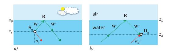
Figure 1: Model for the source ghost (a) and receiver ghost (b).
