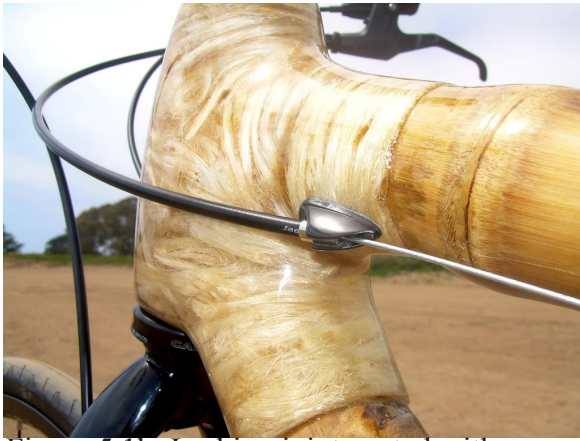
Figure 5.1b: Lashing joint coated with epoxy resin. Figure 5.1c: Rope passed through slotted bamboo
