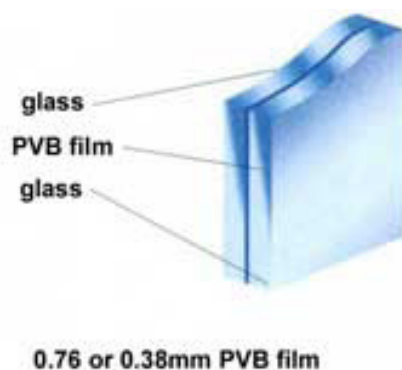
Figure 5.2c: Lamination with PVB film
