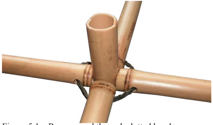
Figure 5.1b: Lashing joint coated with epoxy resin. Figure 5.1c: Rope passed through slotted bamboo
