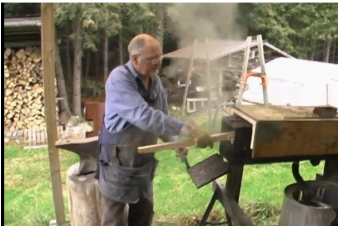
Figure 6.1d: Bamboo cured in steam box.
