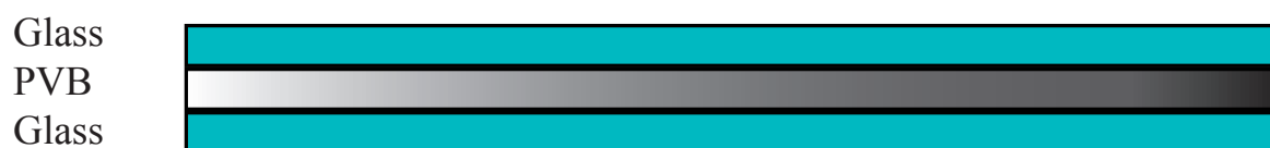
Figure 13.1a: Double layer glass with PVB interlayer
