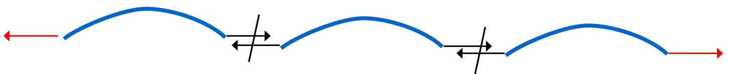
Figure 14.7e: Reaction force of last panel is considered. Reaction forces of in between panels will negate each other.
