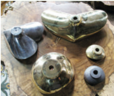
Figure 5.1n: Metal end supports, Marcelo Villegas
