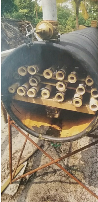
Figure 11.4d: Bamboo steaming for bending. ref: 24H Architect
