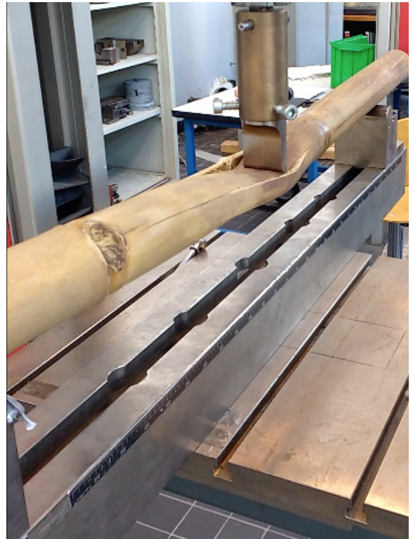
Figure 11.4c: Failure in specimens with length less than 26D.
