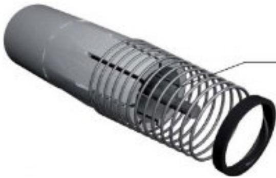
Figure 14.8b: Bamboo sliced and tapered using aluminium ring (Val, 2011).
