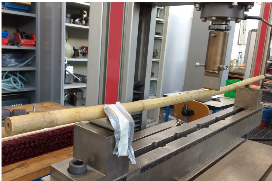
Figure 11.3h: 3-point bending test of bamboo length 920mm and diameter 50mm.
