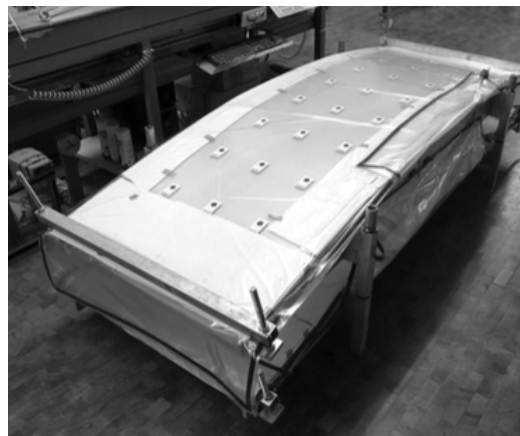
Figure 6.2b: Cold Bending of laminated glass in vacuum using aluminium mould ref: (Fildhuth, 2015)
