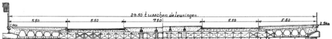
Figure 2-5: Cross section Leiden Bridge
