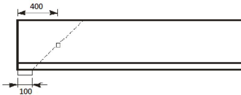
Figure 3-8: Location of first crack
