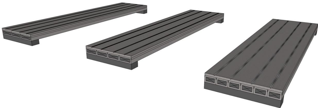
Figure 9-12: Section variants, from right to left: B=1000, 1500 and 2000mm
