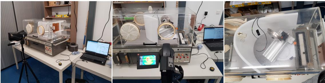
Figure 4.16: Experimental setup to determine the directional dependency of the emissivity of a lithography lens.
