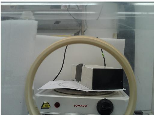
Figure 4.18: Experimental setup to measure the directional dependency of the emissivity.
