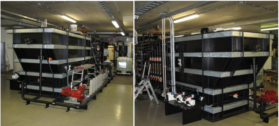
Figure 2. Setup of the one-stage partial nitritation/anammox pilot reactor used for the experimentation.
