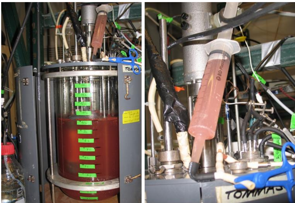
Figure 12. Syringe connected to the reactor mixed liquor by means of which the biomass settling properties were monitored.
