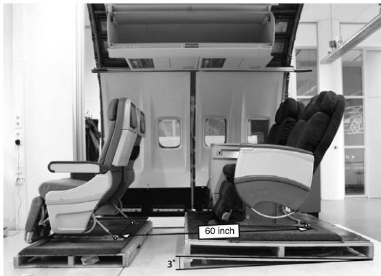
Fig. 2. Inclination angle and pitch length.
