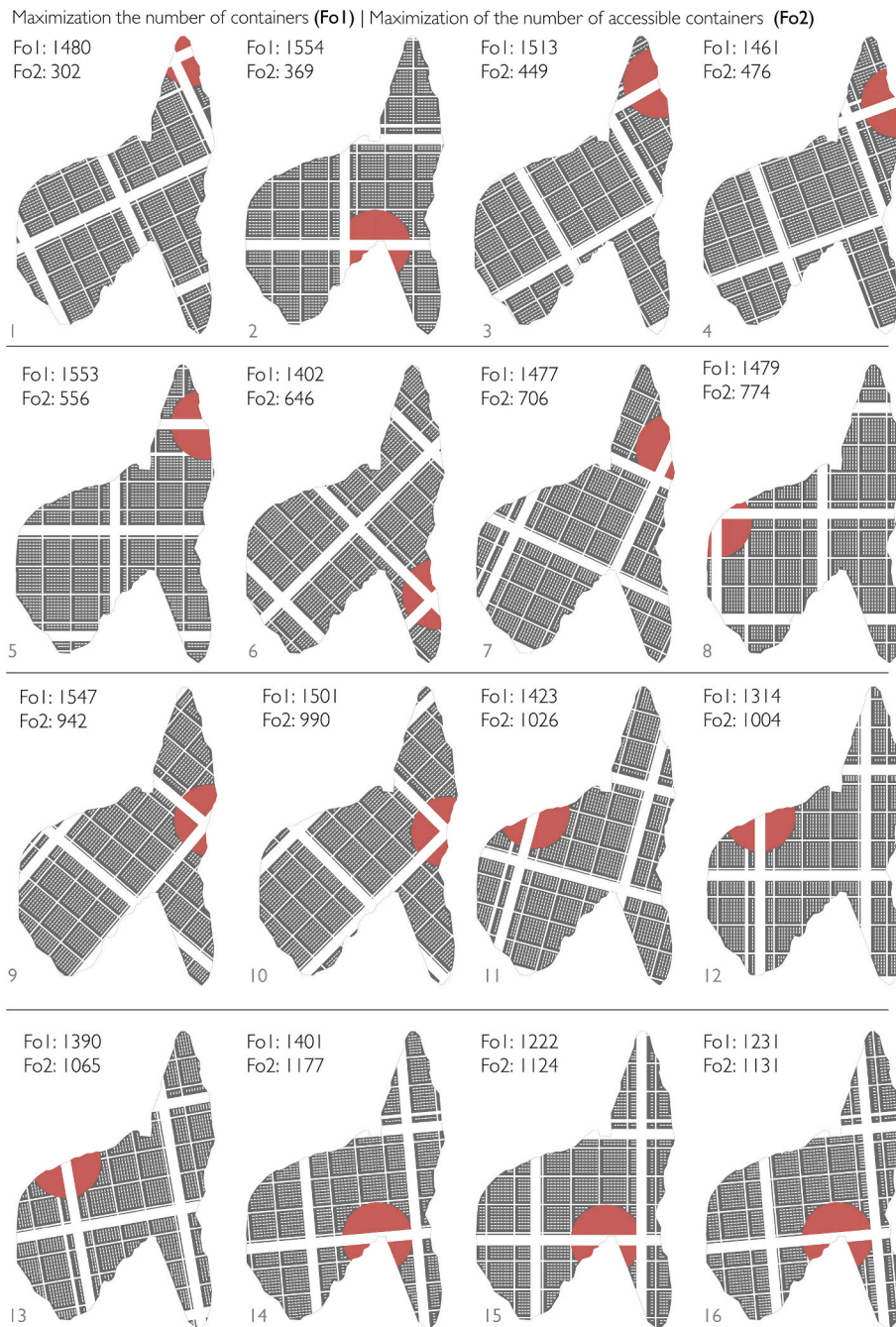
Fig. 5. Sixteen Pareto-optimal solutions arranged by increasing accessibility. Each cell displays site layout with performance metrics. Red indicates service areas, white indicates individual shelter units, and grey indicates shelter blocks/clusters. (For interpretation of the references to colour in this figure legend, the reader is referred to the web version of this article.)
