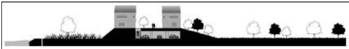
Figure B-6: Cross section with infrastructure and car parking inside the dike and housing on the dike
