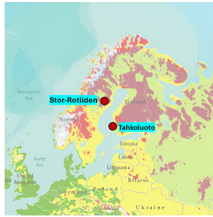
Figure 4.4: IEA Ice Class map showing Ice Classes I-III. Green → I, Yellow → II, Red → III. Stor-Rotliden is located in an Ice Class III region. (VTT Technical Research Centre of Finland, 2015)
