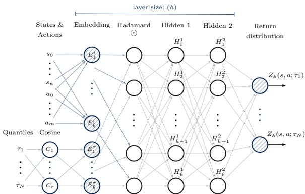
Fig. 9. Depiction of the implicit quantile network (IQN) based on Dabney et al. (2018), with 2 hidden fully-connected feed-forward layers of size  $\bar{h}$ , cosine embedding layer size  $C$  and  $N$  generated quantiles fractions.
