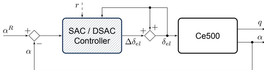
**Figure 4.5:** RL architecture to control the angle of attack of the Ce500 LTI model.
