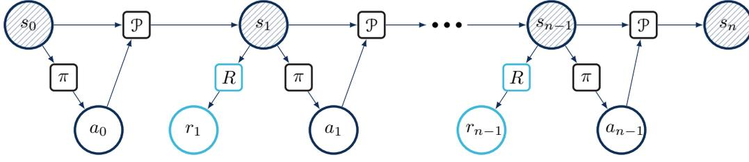
**Figure 3.2:** Depiction of the MDP following policy  $\pi(a | s)$ , with Markov Process  $\langle \mathcal{P}, R \rangle$ .
