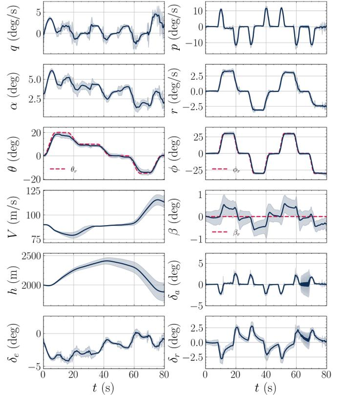
Fig. 14. Evaluation of SAC agents trained using the baseline observation  $s_1$ . Red dashed lines show the reference signals, solid blue lines show the mean response and the shaded areas show the 95% confidence interval.
