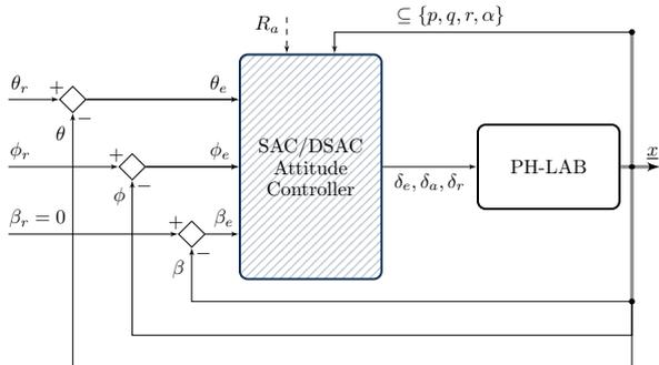
Fig. 7. SAC/DSAC attitude controller architecture with direct deflection control  $a = \underline{u} = [\delta_e, \delta_a, \delta_r]^T$ .
