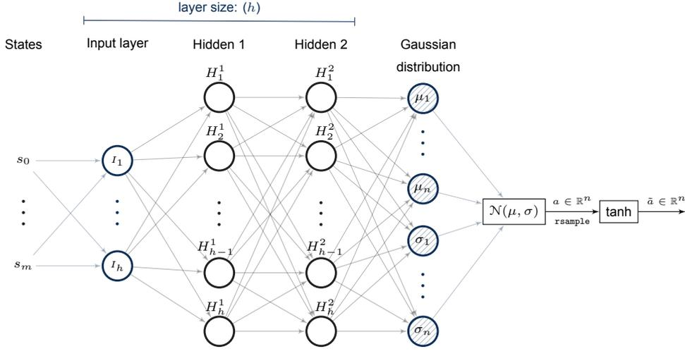
**Figure 3.10:** Depiction of the  $m$ -dimensional multivariate tanh-Gaussian stochastic policy network used by the SAC algorithm.
