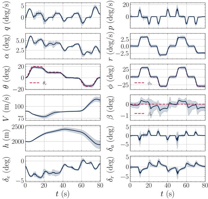
Fig. 15. Evaluation of risk-averse DSAC agents trained using the augmented observation  $s_2$ . Red dashed lines show the reference signals, solid blue lines show the mean response and the shaded areas show the 95% confidence interval.
