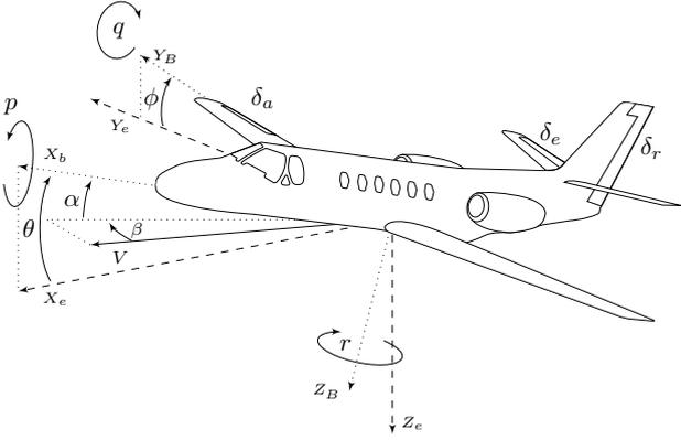
Fig. 6. Visualization of the dynamic states of the aircraft, where  $X_b$ ,  $Y_b$  and  $Z_b$  define the body frame with attitude  $[\phi, \theta, \psi]$  relative to the inertial frame. The heading  $\psi$  is depicted as zero for visual clarity.
