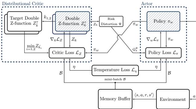
Fig. 5. Distributional Soft Actor-Critic (DSAC) architecture with adaptive temperature and risk-sensitive learning.
