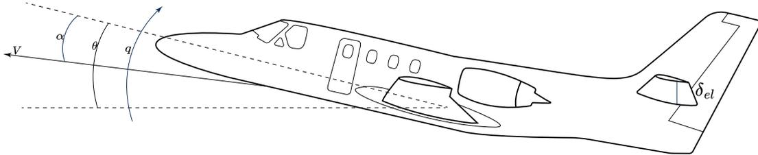
**Figure 4.2:** Cessna 500 (Ce500) short period model with two states: angle of attack (a.o.a)  $\alpha$  and pitch rate  $q$ . The control input is the elevator deflection  $\delta_e$ .
