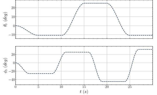
Fig. 8. Pitch  $\theta_r$  and roll  $\phi_r$  reference signals for training are randomly generated sequences of cosine smoothed steps, shown for a single episode.
