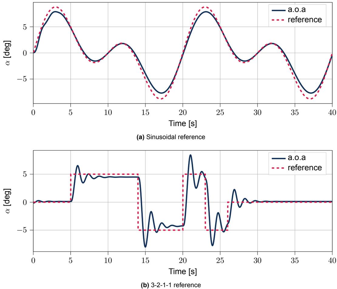
**Figure 4.11:** DSAC post-training control tracking performance evaluation.
