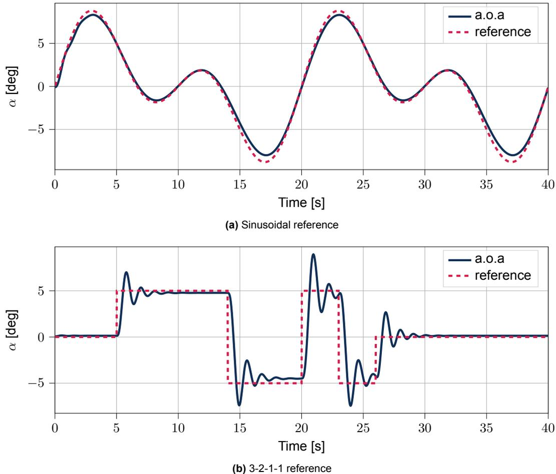
**Figure 4.10:** SAC post-training control tracking performance evaluation.
