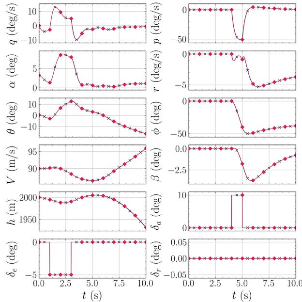
**Figure 6.1:** Pulse response of the simulated PH-LAB environment (red diamond markers) and the original DASMAT Simulink environment (dark cross markers) show identical trajectories.
