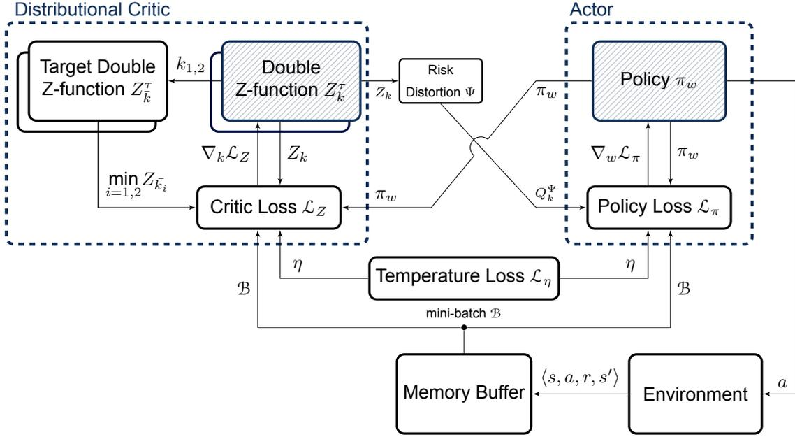
**Figure 3.14:** Depiction of the distributional SAC (DSAC) algorithm architecture.
