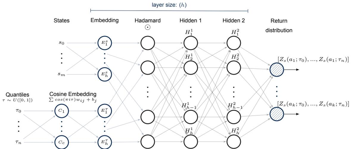
Figure 3.12: Depiction of the implicit quantile network (IQN) based on [31].
