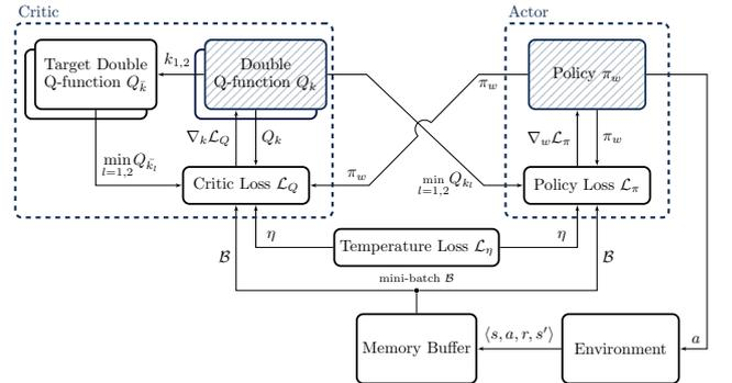
Fig. 1. Soft actor-critic (SAC) architecture with adaptive temperature  $\eta$  optimization and double critic soft Q-networks.
