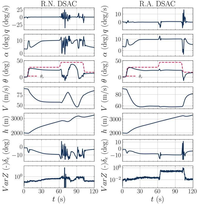
Fig. 18. Comparison of near-stall attitude control task of risk-neutral (left) and risk-averse (right) DSAC controllers; augmented observation  $s_2$ ; Risk-averse trained using Wang(-2.0); Red dashed lines show the reference signals.
