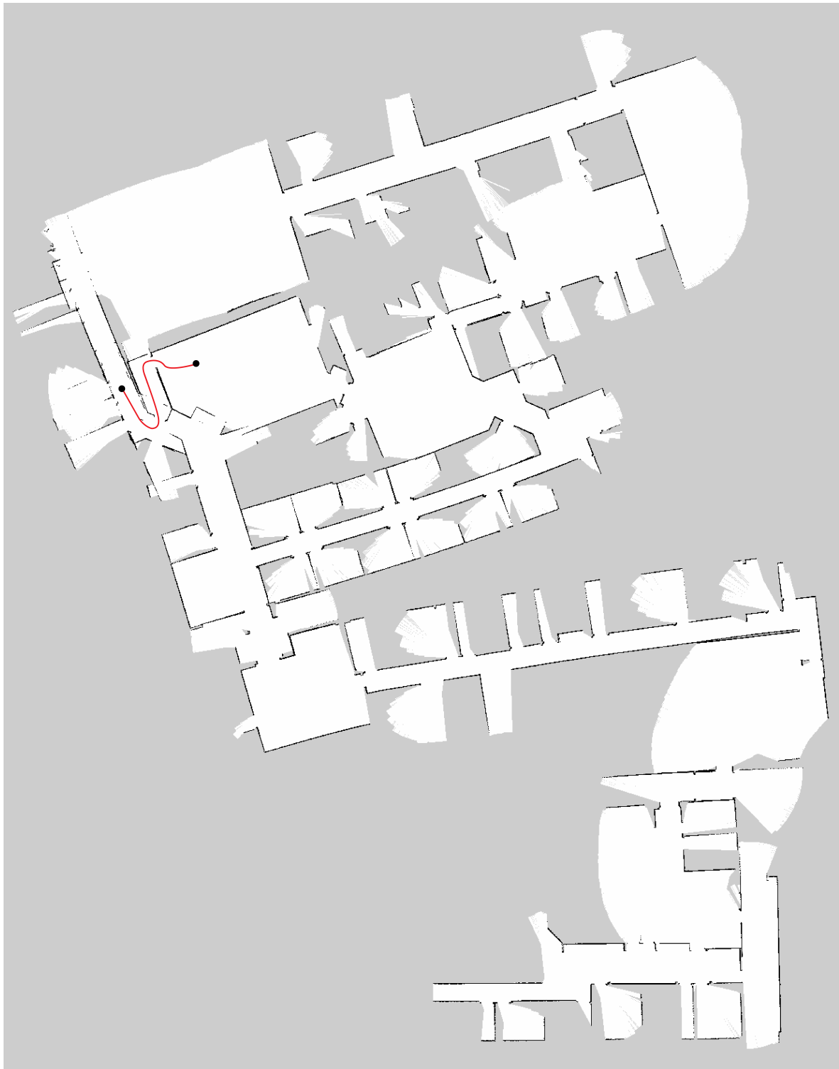
Figure 5-11: Maps constructed in the large scale mapping experiment: baseline system. The red line is a realistic path that a metric planner could come up with when planning between the black dots. This path is impossible to travel however, resulting in failing metric navigation.
