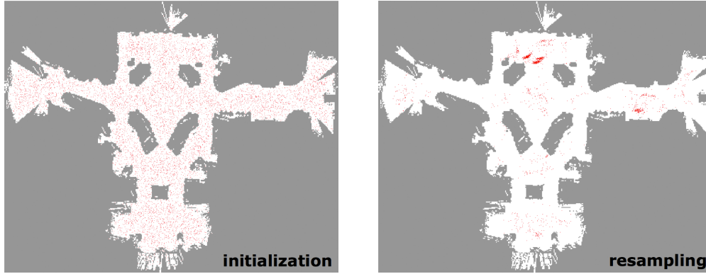
Figure A-9: Left: Initial sample distribution for determining robot location in a known map. Initially nothing is known about the robots location. Right: After a few motion updates and measurement updates from the robot, resampling could lead to such a sample distribution. Figures adopted from [Stachniss, 2013].
